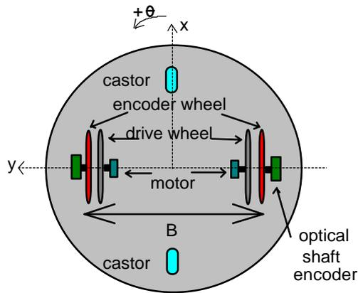
Figure 4 : The odometry system.
