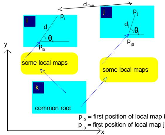
**Figure 10 : Illustration of the computation of the standard deviation of  $d_{min}$**
