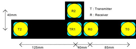
**Figure 3: The sonar array configuration.**
