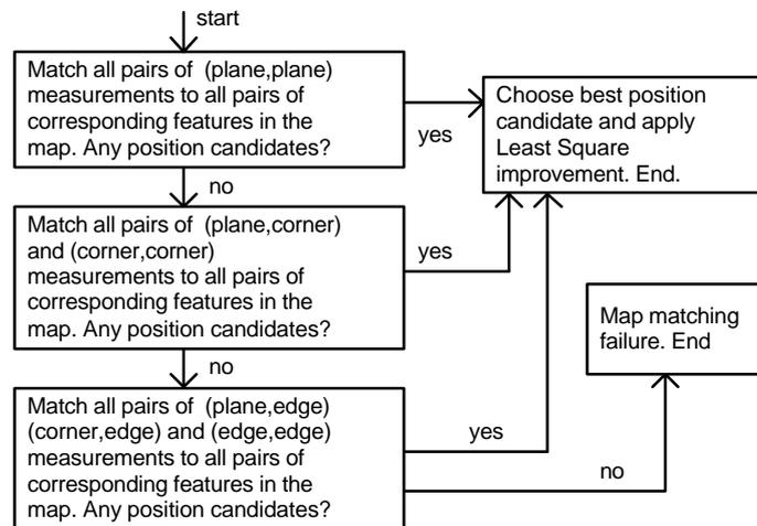
**Figure 6 : Simplified map matching algorithm based on the reliability of features.**
