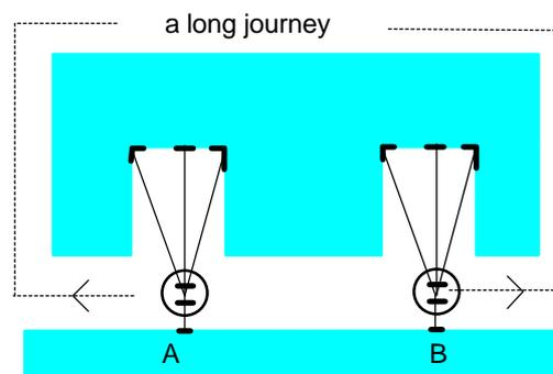
**Figure 13 : The robot at position B has mistaken that it is back to location A after a long journey due to the similarity in observed landmarks at both positions, hence it loads the corresponding previous local map and performs a successful map match due to its large position covariance.**
