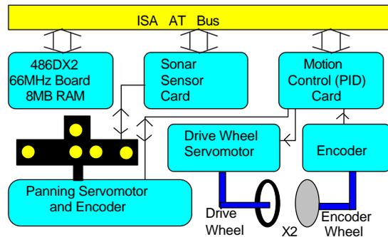
Figure 5 : The robot system architecture.
