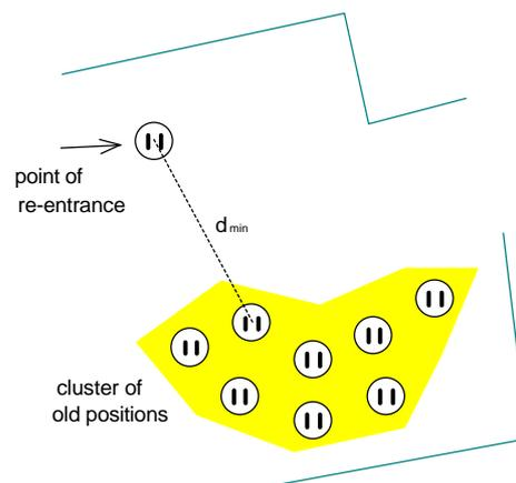
**Figure 12 : The robot enters a previous local map but the algorithm fails to try map matching with this local map because  $d_{min}$  is too large.**
