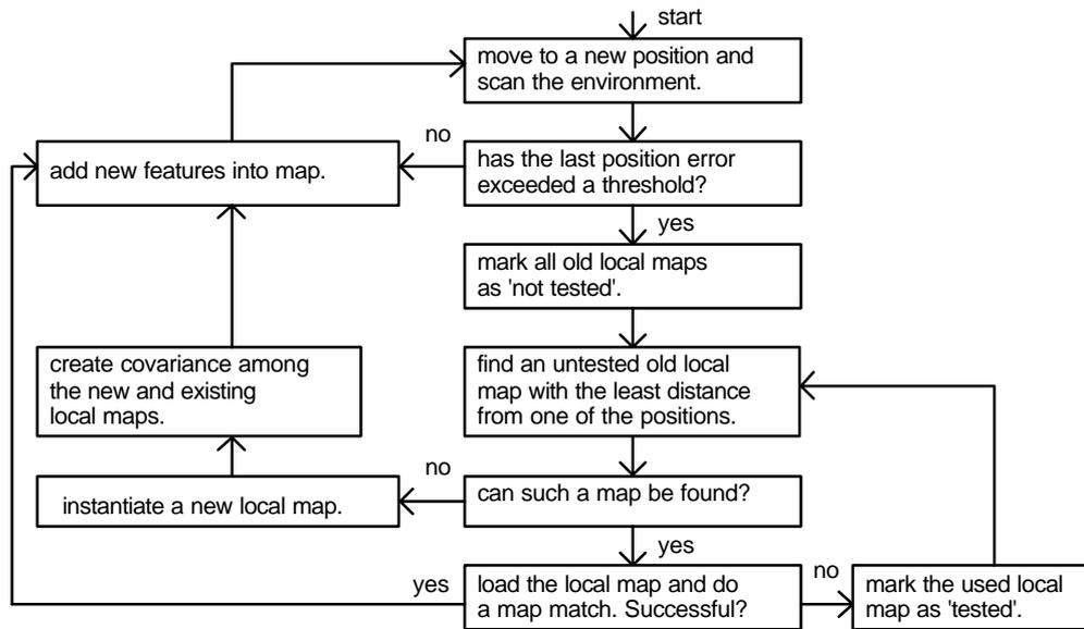
**Figure 8 : Flowchart for the local mapping algorithm.**
