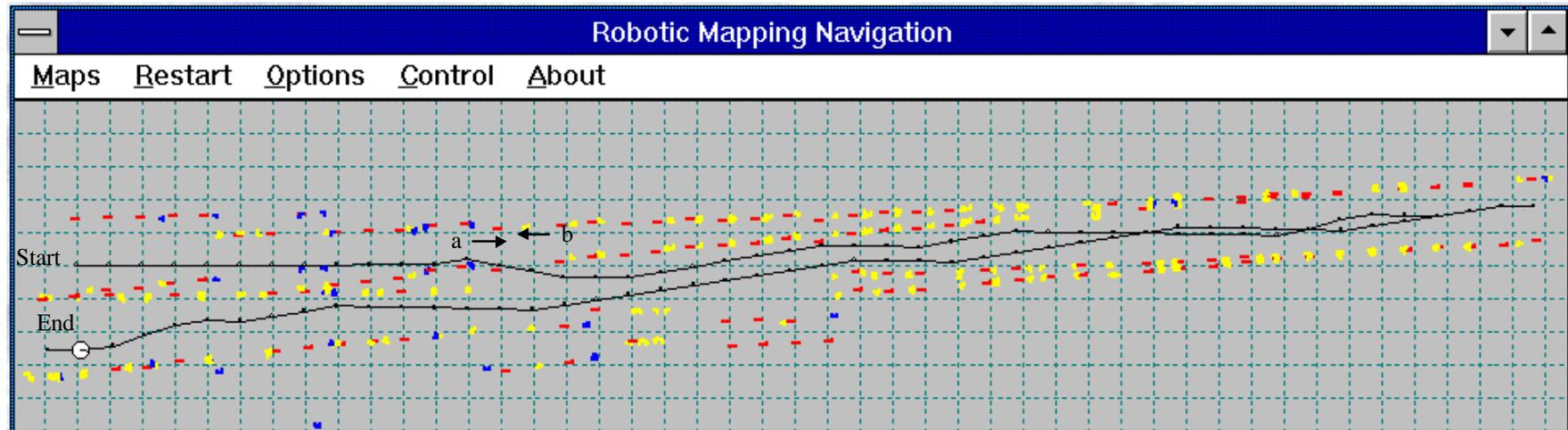
Figure 14 : Raw sonar data for the long corridor experiment (views 'a' and 'b' are shown in Figure 15)
