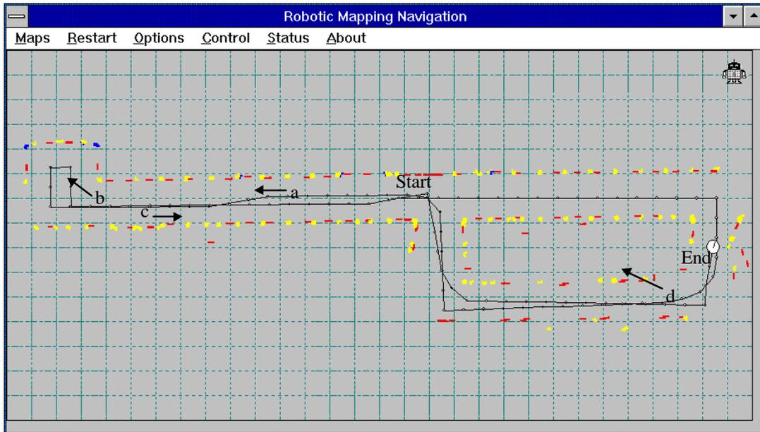
Figure 19 : Raw sonar data for the lab loop experiment (views 'a' - 'd' are in Figure 20).
