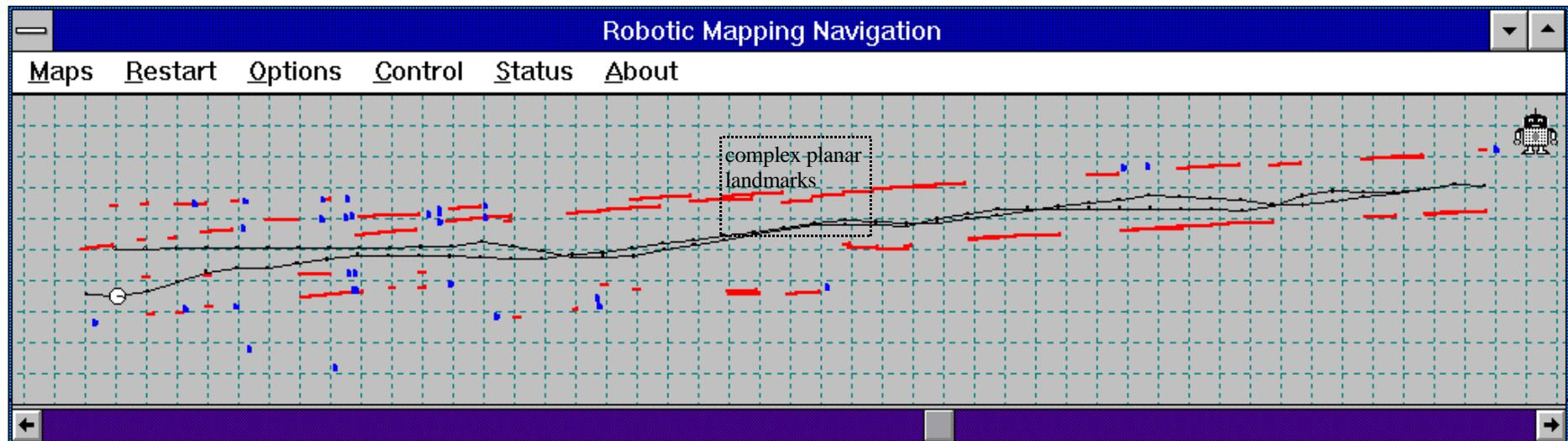
Figure 16 : Global mapping using plane and corner measurements only, for the long corridor experiment
