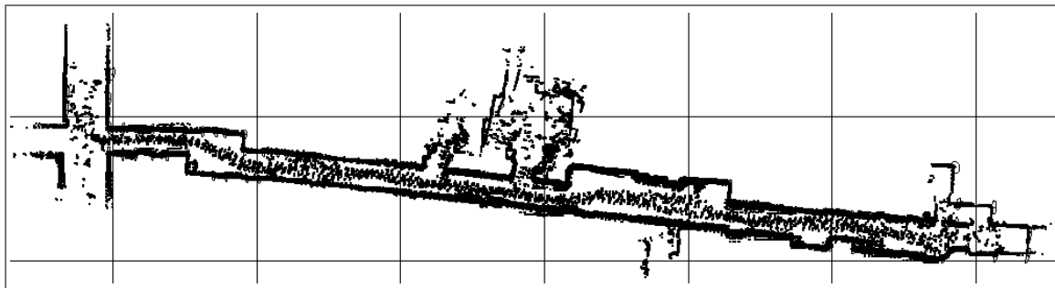
Fig. 7. Registered laser scans overlaid on corrected robot path.
