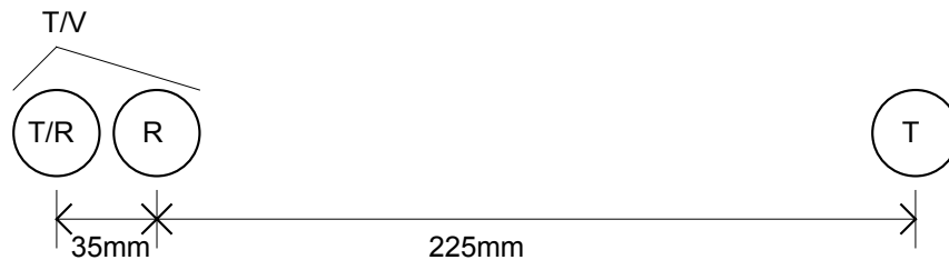
Figure 8 - Sensor arrangement, T=transmitter R=receiver V=vector receiver.
