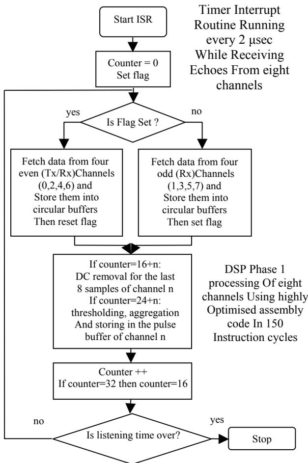
Figure 4. Phase one real time processing flow chart
