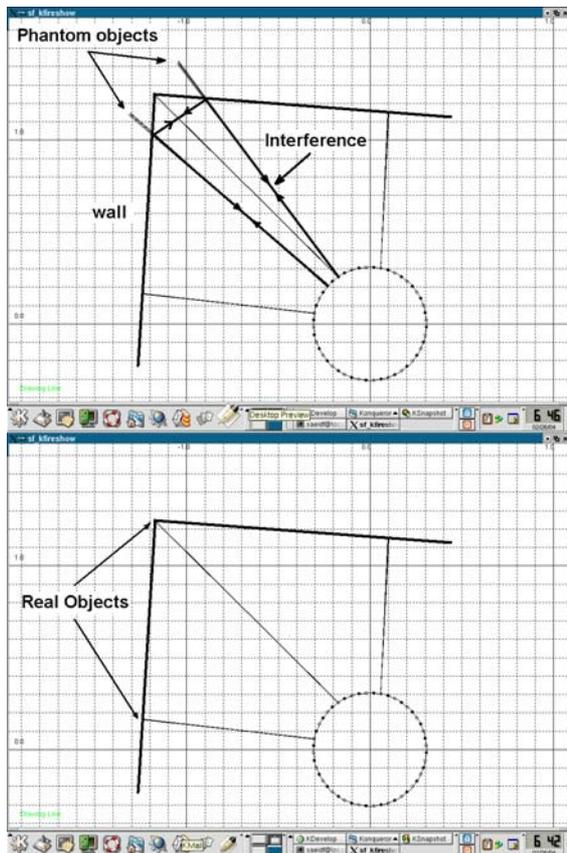
Figure 7. Target association results before and after applying interference rejection idea
