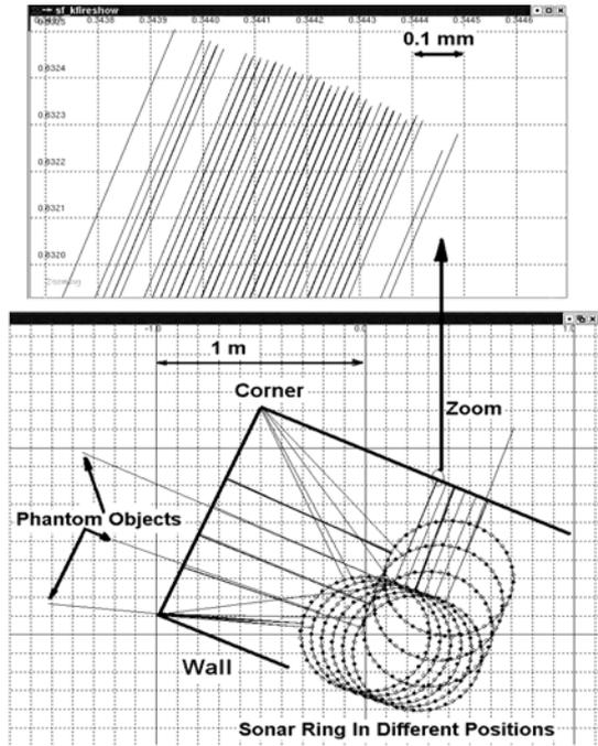
Figure 5. Targets associated by advanced sonar ring in the real environment
