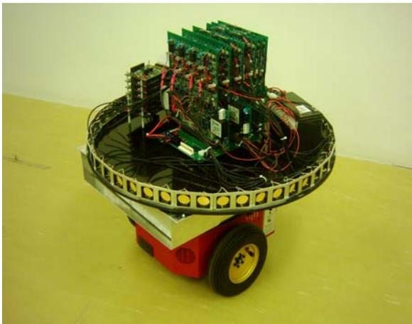
Figure 1. Advanced sonar ring mounted on an ActivMedia Pioneer 3 DX mobile robot.
