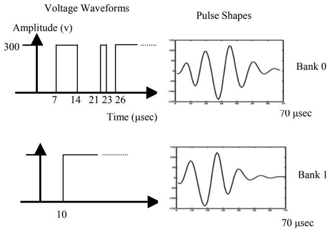
Figure 6. Voltage waveforms used to drive transmitters and echo pulse shapes of bank 0 and bank 1
