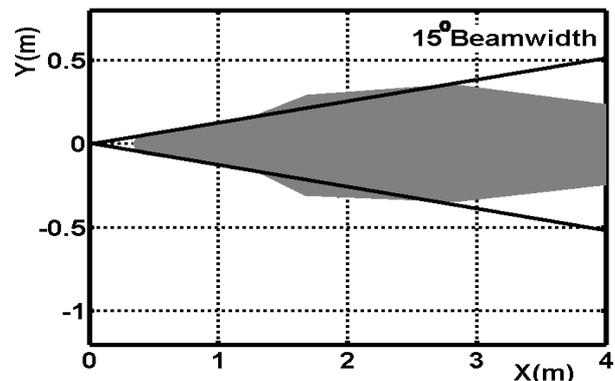
Figure 2. The measured beamwidth of a pair of transducers in gray – the solid line indicates the requirement for the ring to cover 360 degrees.
