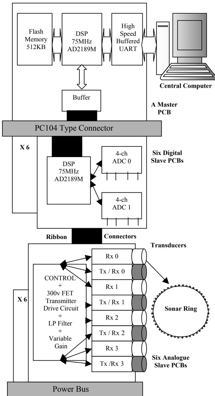
Figure 3. Advanced sonar ring hardware block diagram
