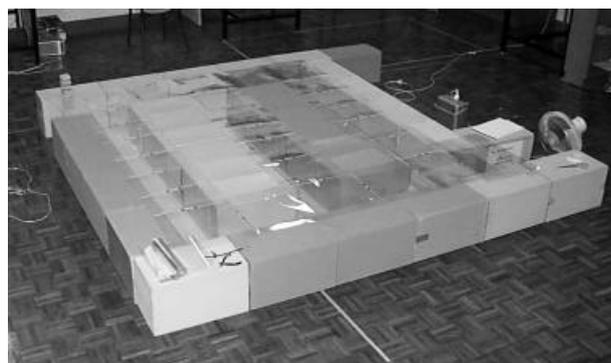
Figure 5 The experimental environment - a simple maze with induced airflow.
