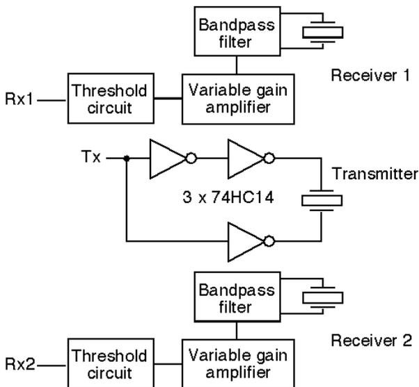
Figure 1 A block diagram of the ultrasonic sensor.
