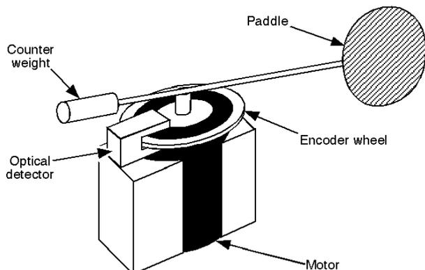
Figure 3 The main components of the airflow sensor.
