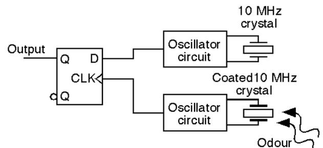
Figure 2 Quartz crystal microbalance sensor circuit.
