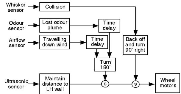
Figure 7 Proposed control scheme for the rescue robot.
