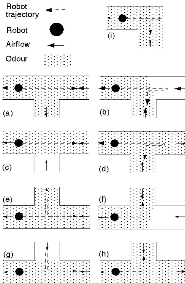
Figure 6 The different situations encountered by the rescue robot.
