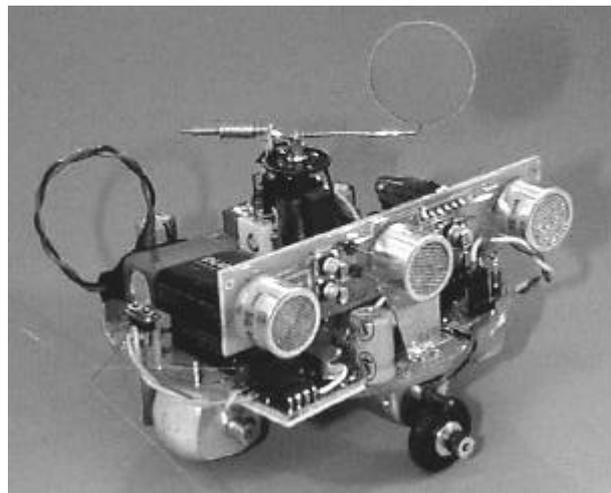
Figure 4 The rescue robot: a RAT robot equipped with ultrasonic wall-following sensors, an airflow sensor, whisker bump sensors, and a chemical sensor.
