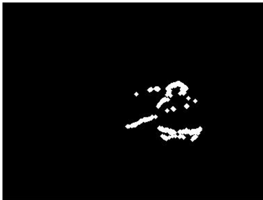
Figure 9. Difference pixels from subtraction of successive frames highlights movement (here, the mouse pad and the author's arm).
