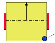
Associate new measurement to corner feature Constrains robot position and orientation
