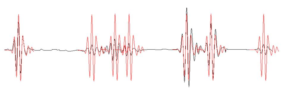
Templates shifted to best match the pulses using correlation of the template with the pulse. Shape (not amplitude) are matched by a correlation.
