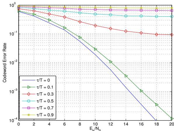
Fig. 8. Impact of time delay on codeword error rate for QPSK Golden code without knowledge of  $\tau$
