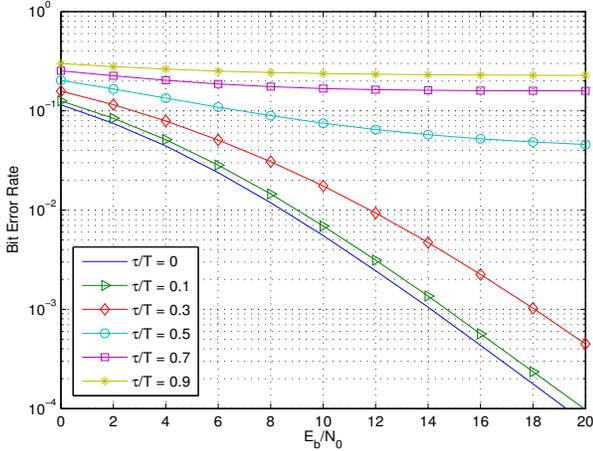
Fig. 4. Impact of time delay on bit error rate for BPSK Alamouti scheme using symbol by symbol Alamouti detection
