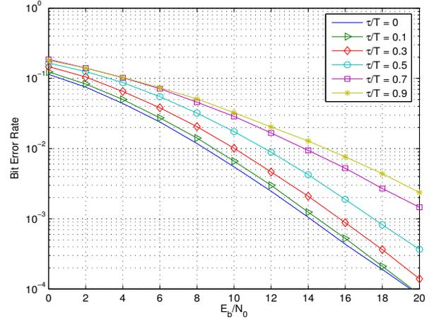
Fig. 6. Impact of time delay on bit error rate for BPSK Alamouti scheme using ML detection with ideal DFE
