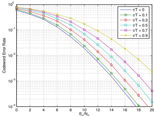
Fig. 7. Impact of time delay on codeword error rate for QPSK Golden code with knowledge of  $\tau$
