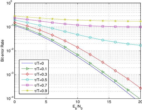
Fig. 5. Impact of time delay on bit error rate for BPSK Alamouti scheme using symbol by symbol Alamouti detection with ideal DFE
