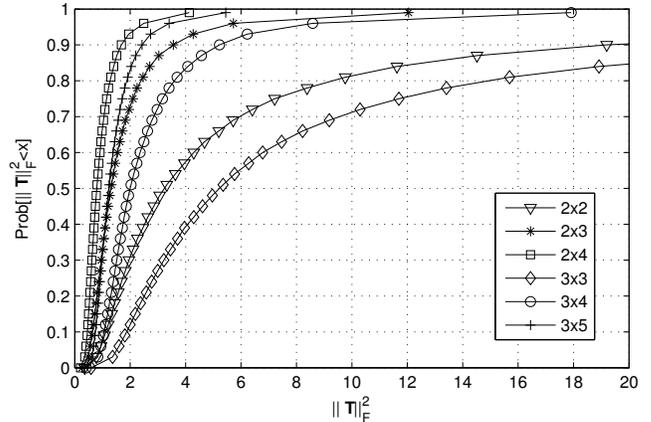
Fig. 2. C.d.f. of the power enhancement with beamforming
