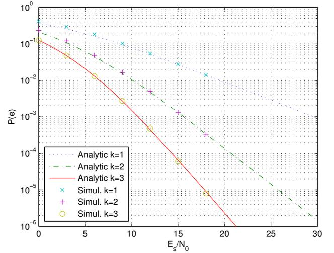
Fig. 5. Effects of error propagation on the error probability of each user with QPSK
