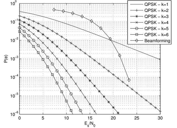
Fig. 4. Error probability of each user with QPSK compared to ZF beamforming
