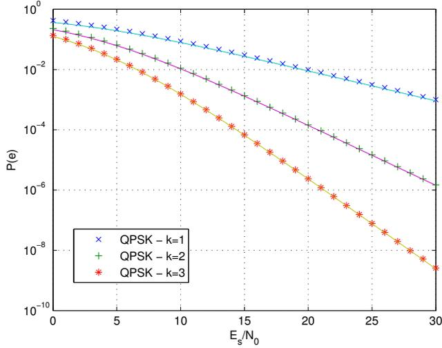
Fig. 3. Error probability of each user with QPSK: comparison of exact expressions (continuous lines) and upper bounds (markers)
