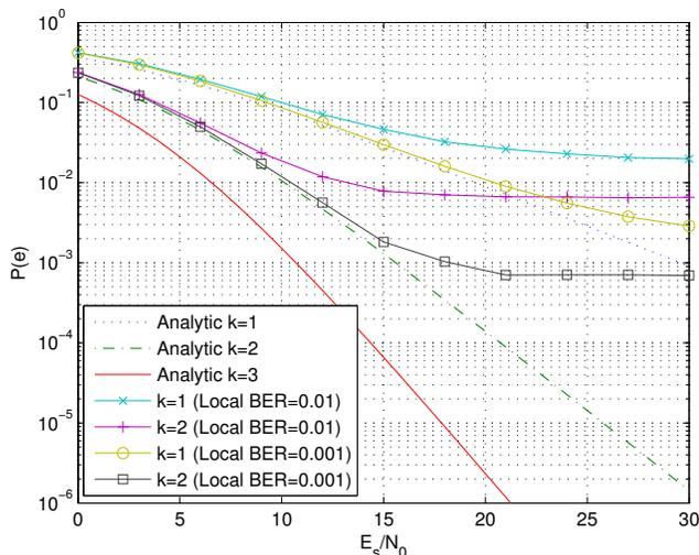
Fig. 6. Effects of local channel errors on the error probability of each user with QPSK
