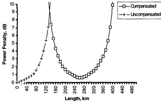
Fig. 4: Power penalty due to dispersion versus fiber length
