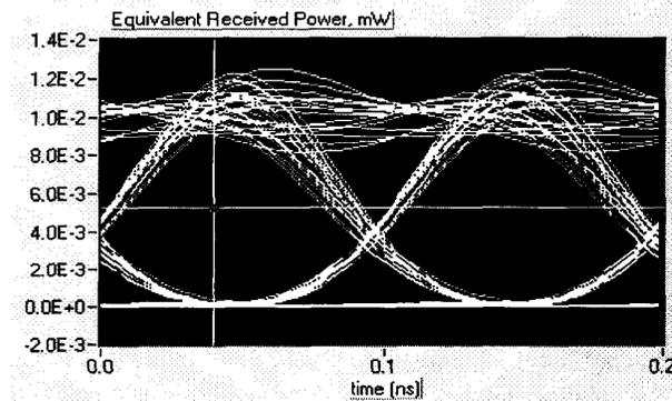
Fig.5: Eye diagram for a 270-km compensated system with the optimum sampling point indicated
