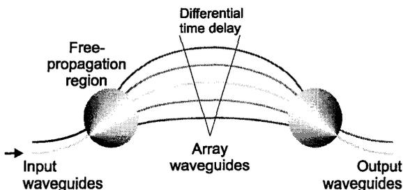
*Figure 1: Simplified schematic of an AWGM/AWGR showing the distribution of power from the active Input Waveguide (arrowed) to the Array Waveguides, which act as delays. If the AWGM is unchirped, the outputs of the Array Waveguides will constructively interfere at one Output Waveguide at frequencies separated by the free spectral range.*
