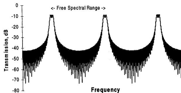
Fig. 2: 121-Guide AWGM response with Gaussian power distribution and chirp
