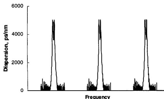
Fig. 3: Dispersion that can be compensated (ps/nm) by the AWGM versus optical frequency. Free spectral range = 200GHz.
