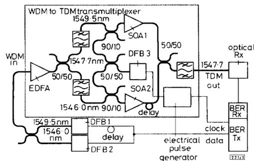
Fig. 1 Experimental configuration
