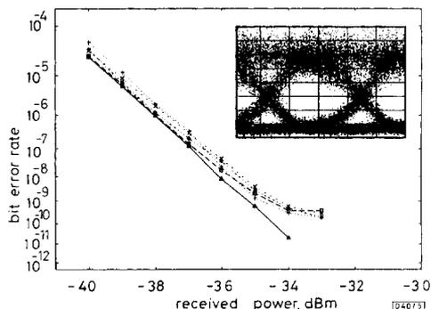
Fig. 5 Measured bit error rates and eye diagram at 622Mbit/s
