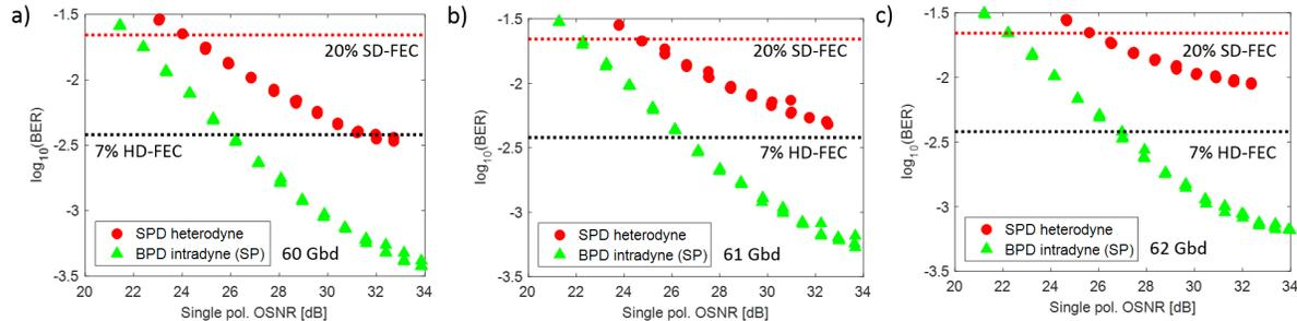
Fig. 3: Back-to-back performance results, with signals modulated at a) 60, b) 61 and c) 62 Gbd. Red circles are for dual-polarization measurement with the heterodyne receiver, green triangles for single-polarization intradyne reception. Indicative thresholds for a 7% HD FEC and 20% SD FEC are shown in dotted lines.
