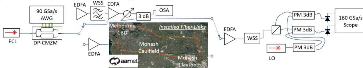
Fig. 2: Experimental set-up for the single photodiode-per-polarization receiver trials. EDFA: erbium doped fiber amplifier, OSA: optical spectrum analyzer, WSS: wavelength selective switch, (PM) 3dB: (polarization maintaining) 3 dB coupler.
