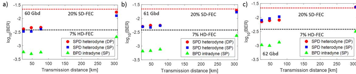
Fig. 4: Transmission performance at optimum launch power (6 dBm) over various distances of field-installed fiber with a) 60, b) 61 and c) 62 Gbd signals received. Red circles represent dual-polarization heterodyne reception, blue squares for heterodyne reception of a single polarization signal, and green triangles intradyne reception of a single polarization signal. Indicative HD and SD FEC thresholds are shown in dotted lines.
