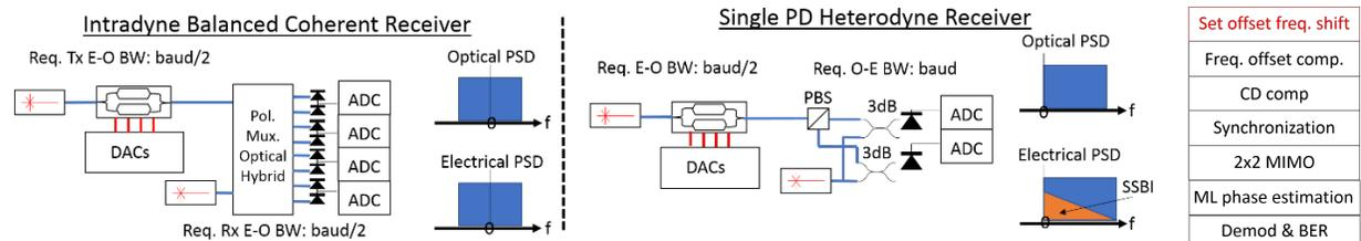
Fig. 1: Basic architecture of (left) intradyne and (middle) single photodiode heterodyne receivers. The insets compare the received power spectral densities (PSDs) of the optical and electrical signals. (right) Receiver DSP flow for the intradyne and heterodyne systems. These are identical, excepting the frequency shift stage at the start of the heterodyne Rx DSP (red).
