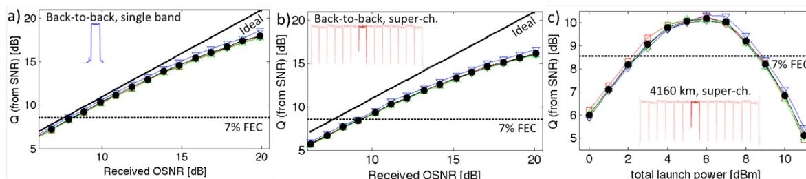
**Fig. 3:** Performance under noise loading of an fOFDM band as a) a single band and as b) the centre band within a super-channel. c) Performance of the fOFDM band after 4160-km super-channel transmission at varied launch powers. Solid black lines give ideal performance, open markers individual sub-carrier values and solid markers the mean values for the measured band. Dashed lines: 7% hard-FEC threshold.
