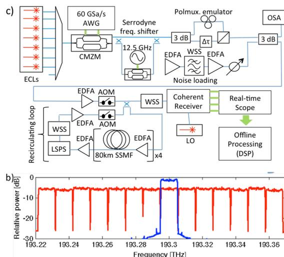
**Fig. 2** –a) Measured spectrum of the generated 14-band fOFDM superchannel; b) Experimental set-up. ECL: External cavity laser, LSPPS: Loop synchronous polarization scrambler, OSA: Optical spectrum analyser, AOM: Acousto-optic modulator, WSS: Wavelength selective switch, CMZM: Complex Mach-Zehnder modulator.
