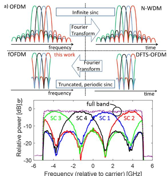
**Fig. 1:** a) Illustration of ‘infinite’ sinc and truncated, periodic sinc fOFDM power waveforms/spectra in N-WDM, OFDM, DFTS-OFDM, for single band signals with four sub-carriers only; b) Measured spectra for each subcarrier and full band of a four sub-carrier fOFDM band.
