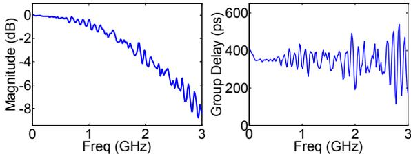
Fig. 3. Measured frequency response (left) and group delay (right) of Mini-circuits SBLP-1870+ LPF.
