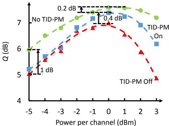
Fig. 4.  $Q$  vs launch power for the center DP-16QAM channel with fitted curves.
