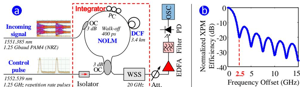
Fig. 1. (a) Experimental setup of noise-resistant optical sampling of 1.25 Gbaud PAM 4 signal; OC: optical coupler; PC: polarization controller; Att.: attenuator; PD: photo-diode; OSC: oscilloscope. (b) XPM efficiency with 400 ps integration time.
