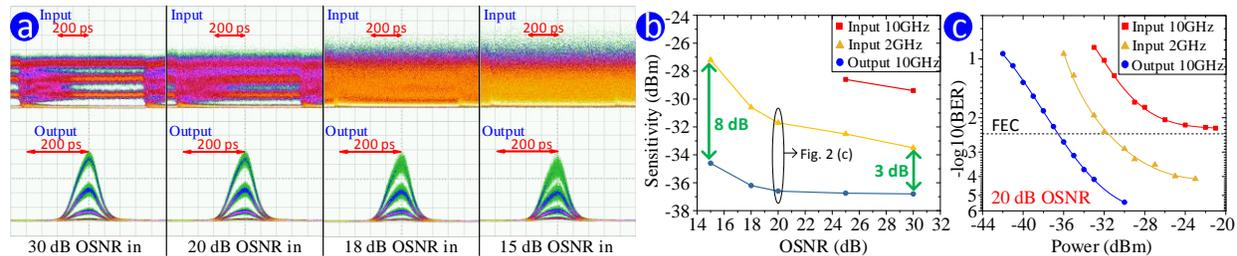
Fig. 2. (a) Eye diagrams of the received signal with 10-GHz anti-aliasing filter and the output of NOLM with 10-GHz anti-aliasing filter under OSNRs of 30 dB, 20 dB, 18 dB and 15 dB. (b) Sensitivity versus OSNR plot (c) BER versus received optical power plot with incoming signal OSNR set to 20-dB, either directly detected with a 2- or 10-GHz anti-aliasing filter, or after NOLM sampling with a 10-GHz anti-aliasing filter.
