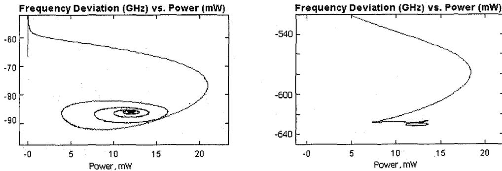
Fig. 2. Turn-on transients of 95%-1% facets (180 deg./ 0 deg.) Bulk (left) and MQW (right) lasers at 60-mA.
