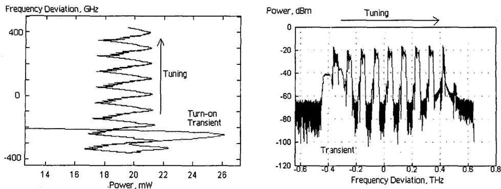
Fig. 4. Phase portrait and time-averaged optical spectrum during tuning of a FP-DBR laser.
