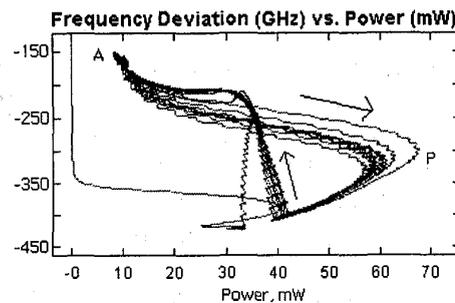
Fig. 3. Phase portrait for a uniform DFB laser driven at 160 mA showing unstable operation.
