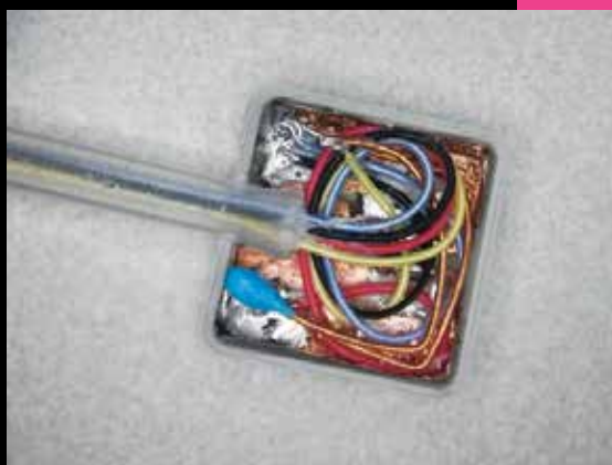
Temperature testing tile used in preclinical experiments to verify that the temperature rise due to wireless transmission of power and data is within safe limits.
