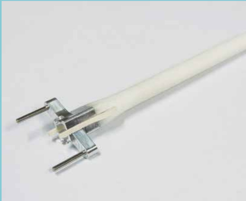
Implant tile handling tool. This tool was custom-designed to avoid damage to the implant tiles and electrodes during assembly and testing.
