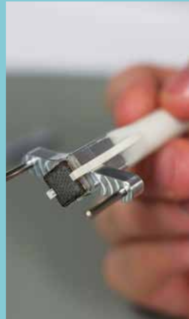
Implant tile handling tool. This tool was custom-designed to avoid damage to the implant tiles and electrodes during assembly and testing.
