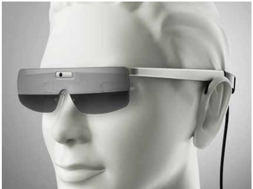
Front and rear perspectives of Gennaris commercial headgear concept. The design has been upgraded to improve usability, including the incorporation of removable lenses (Images courtesy of MADA).
