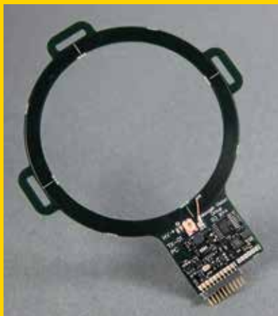
Class E transmitter, including coil and associated electronic circuitry.
