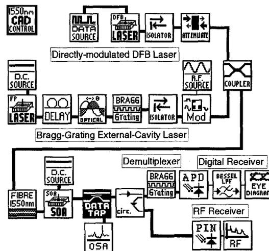
ThG5 Fig. 1. OPALS schematic diagram of a mixed analog/digital system.
