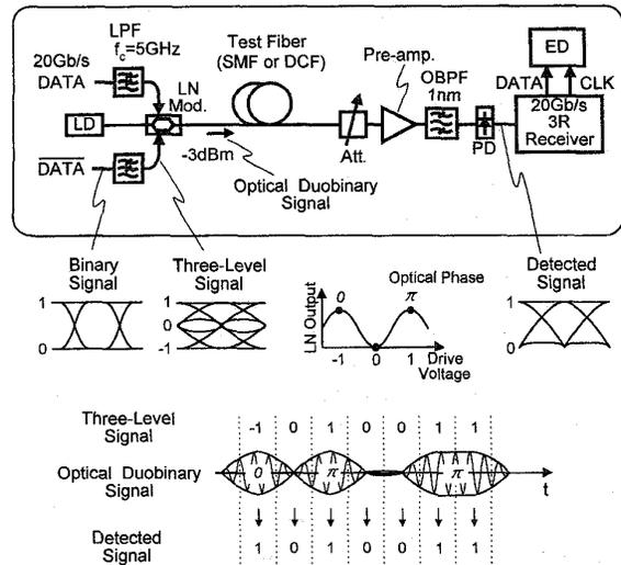
**ThH1** Fig. 1. Experimental setup and corresponding operating conditions for 20-Gbit/s optical duobinary transmission.
