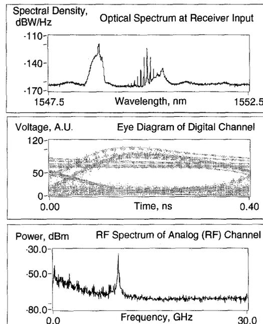
ThG5 Fig. 2. Simulated optical spectrum, eye diagram and RF spectrum showing complex interactions.
