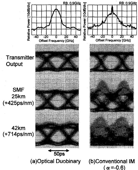
**ThH1** Fig. 2. Measured optical spectra and waveforms for 20-Gbit/s optical duobinary and conventional IM signals before and after transmission over 25 km (+425 ps/nm) and 42 km (+714 ps/nm) SMFs.
