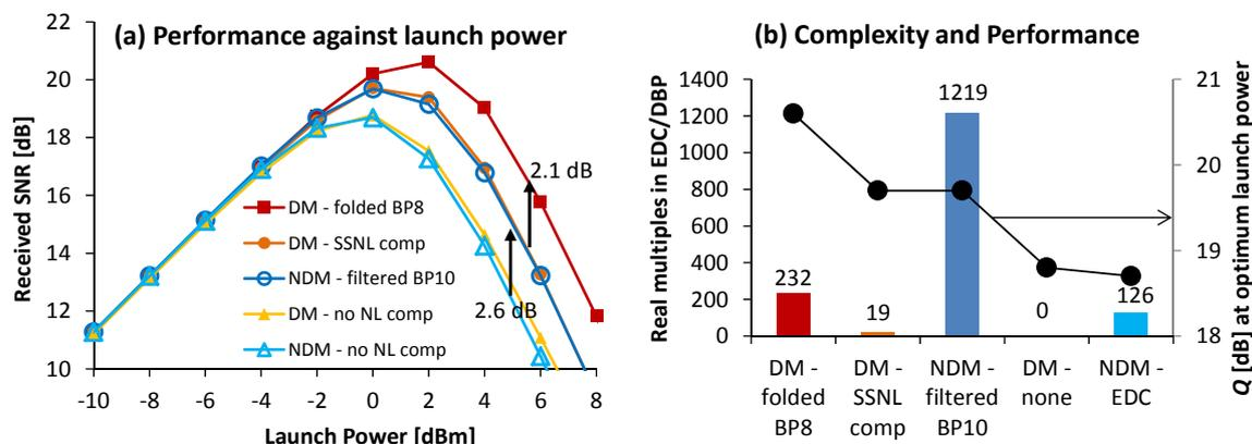
Fig. 3. (a) Received  $Q$  vs. launch power; (b) Real multiplies per symbol for different static equalizers and  $Q$  at optimum power.
