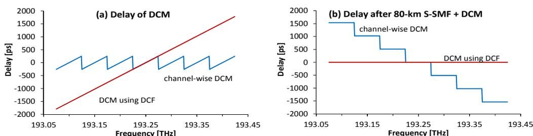
Fig. 1. Relative delays: (a) of 80-km DCM only; (b) of 80-km of S-SMF and 80-km DCM.
