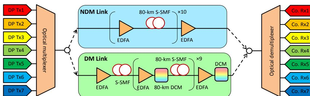
Fig. 2. Simulation setup showing the test and reference links: Co. – coherent.
