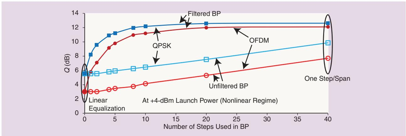
[FIG6] The Q-factor of a 4-QAM 40 × 80-km NDM link with filtered and unfiltered DBP [6].
