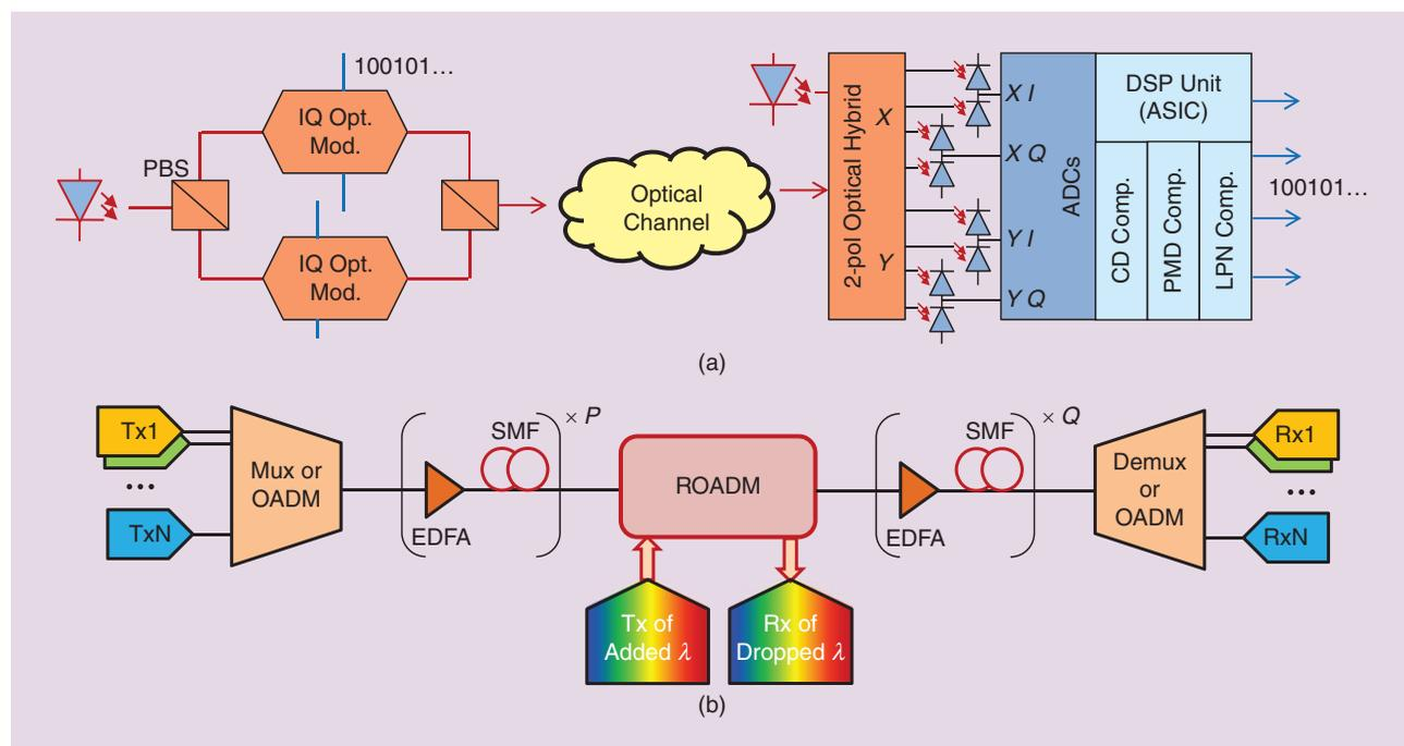
**[FIG1]** (a) The coherent optical transmitter and receiver for current generation 40 Gb/s and 100 Gb/s systems. (b) The conceptual optical link with a single ROADM.
