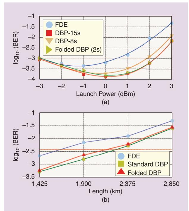
**[FIG5]** (a) Simulation results for a  $10 \times 224$ -Gb/s POLMUX 16-QAM over a  $8 \times 80$ -km DM link. (b) Experimental results for a  $10 \times 111$  Gb/s POLMUX-RZ-DQPSK system at 0-dBm launch power into each span [24].
