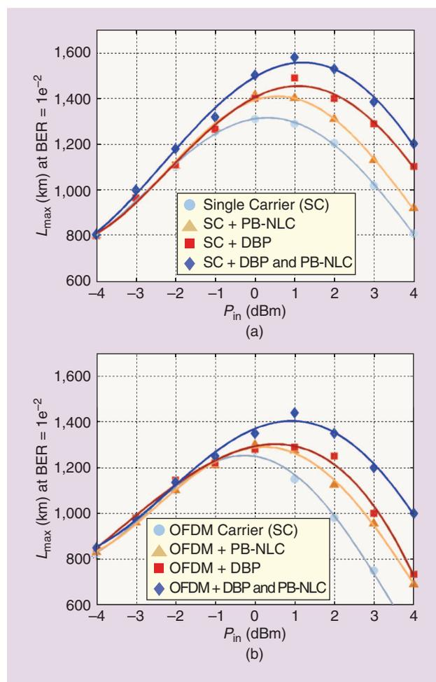
**[FIG8]** The maximum reach distance versus launch power for 9 WDM 16-QAM at 224 Gb/s over an NDM link for (a) single carrier and (b) CO-OFDM [27]. The maximum distance was calculated by assuming a soft-decision FEC with a threshold of  $1.0 \times 10^{-2}$ .
