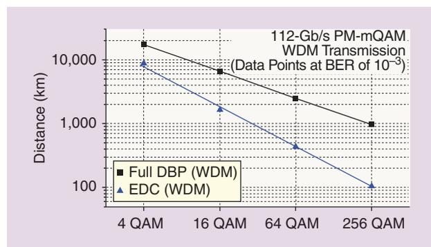
**[FIG3]** The maximum transmission distance at optimal power achieving a BER of  $10^{-3}$  for a WDM system.
