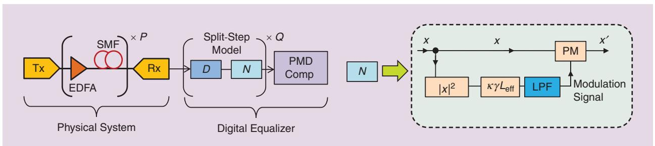
**[FIG2]** An optical system with DBP: dispersion section (D), nonlinear section (N), number of amplified spans in the link (P), number of steps used in DBP (Q), scaling factor to be optimized  $\kappa$ , and phase modulator (PM).
