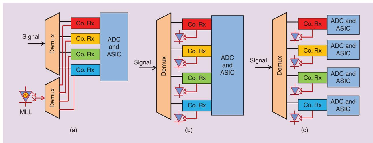
**[FIG10]** Superchannel receiver architectures for a four subchannel system: (a) with a joint ASIC and phase-locked LOs for superchannel DBP, (b) with a joint ASIC and unlocked LOs for coupled-field DBP, and (c) with independent ASICs and coherent receivers for single-channel DBP. *Mode-locked laser* is represented by the acronym MLL.
