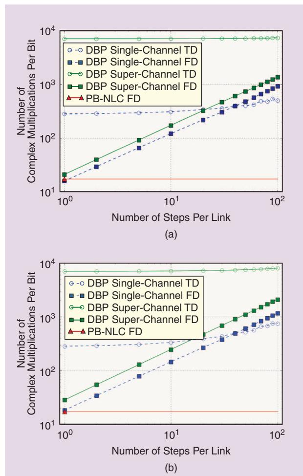
**[FIG9]** The computational cost for PB-NLC and DBP for a given number of steps per link: (a) the conventional unfiltered DBP and (b) filtered digital DBP.
