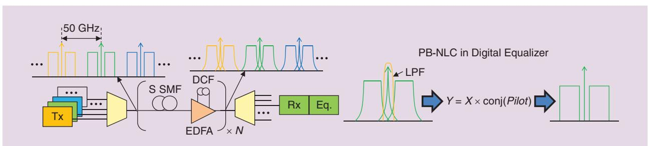
[FIG7] An optical system with PB-NLC.
