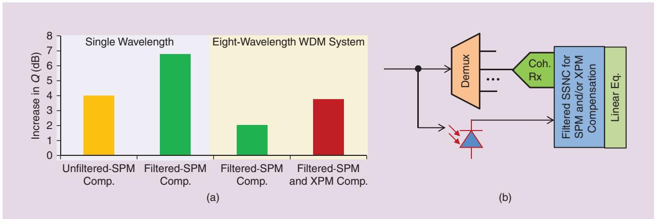
**[FIG4]** (a) The nonlinear threshold increase for 100-Gb/s CO-OFDM in a DM S-SMF link; (b) the SSNC for SPM and XPM compensation.
