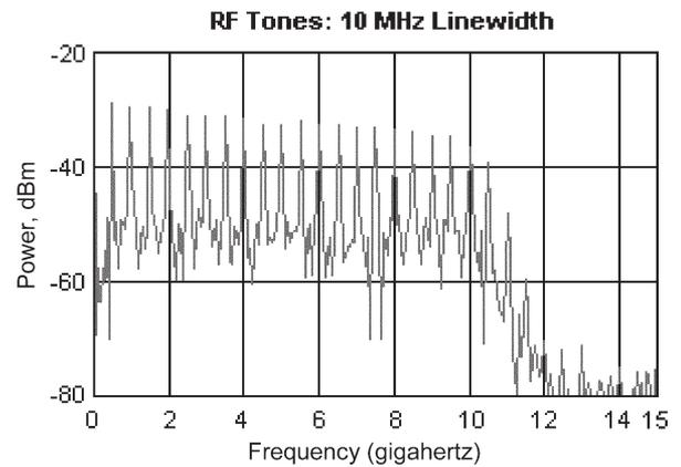
Fig. 10. RF spectrum for a 10-MHz linewidth laser.
