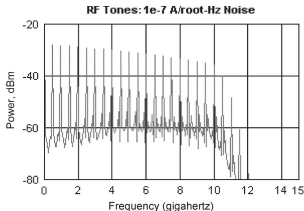
Fig. 17. Effect of electrical noise on the RF tones.
