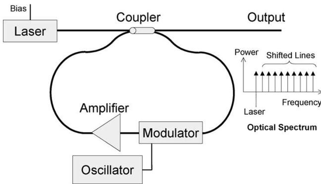
Fig. 2. Optical serrodyne modulator within a loop.
