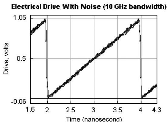
Fig. 16. Sawtooth “eye diagram” showing the magnitude of the electrical noise.
