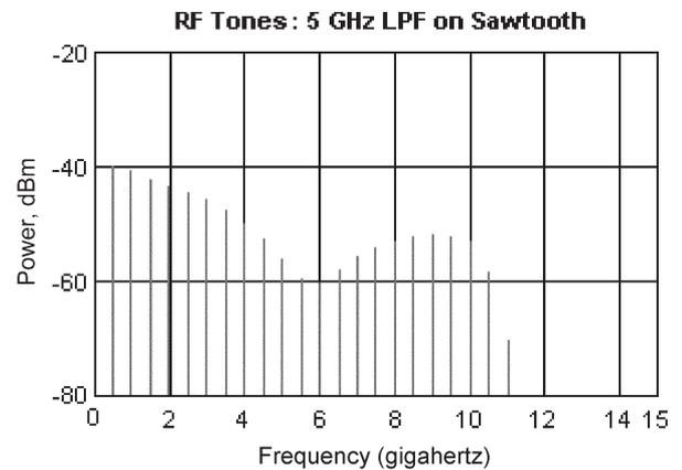
Fig. 15. RF spectrum resulting from the detection of the optical spectrum in Fig. 14.
