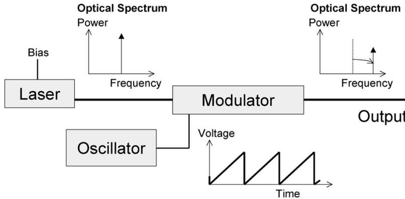
Fig. 1. Optical serrodyne modulation to frequency shift an optical line.
