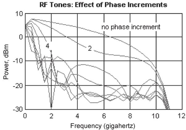
Fig. 20. Effect of incrementing optical phase per circulation (50% couplers). Label is degrees increment per circulation.
