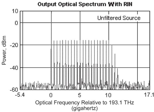
Fig. 11. Optical spectrum for  $-140$  dB/Hz laser RIN.
