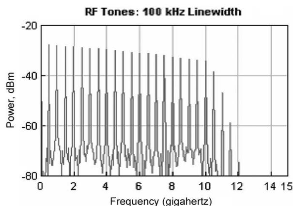
Fig. 9. RF spectrum for a 100-kHz linewidth laser.
