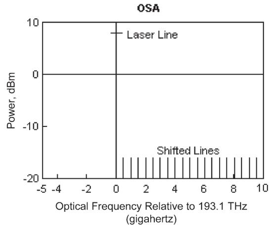
Fig. 6. Optical spectrum after 19 recirculations.
