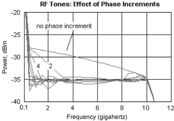
Fig. 19. Effect of incrementing optical phase per circulation (20% couplers). Label is degrees increment per circulation.
