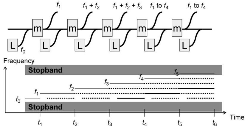
Fig. 3. Unwound model of the loop, where horizontal distance equates to time: L is the source laser (frequency  $f_0$ ); m is the modulator. The optical filter is not shown, but its stopband removes frequency  $f_5$ . The output frequencies are plotted in the graph. The style of the lines indicates the shifting that occurs on each pass of the modulators.
