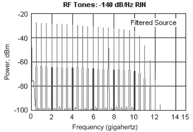
Fig. 13. RF spectrum for  $-140$  dB/Hz laser RIN (filtered source).
