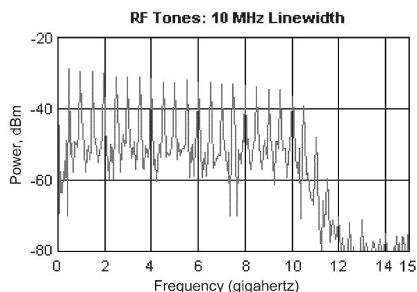
Fig. 10. RF spectrum for a 10-MHz linewidth laser.
