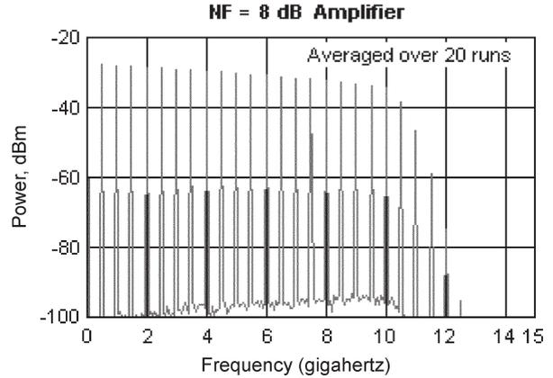
Fig. 21. RF noise due to frequency-shifted optical amplifier noise.
