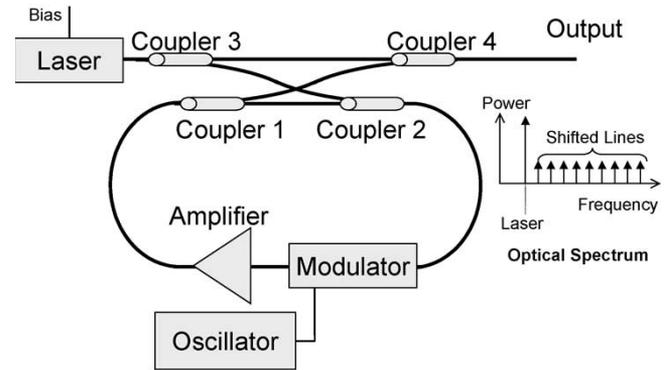
Fig. 4. Optical loop with four three-port couplers to achieve a strong laser line compared with the shifted lines.
