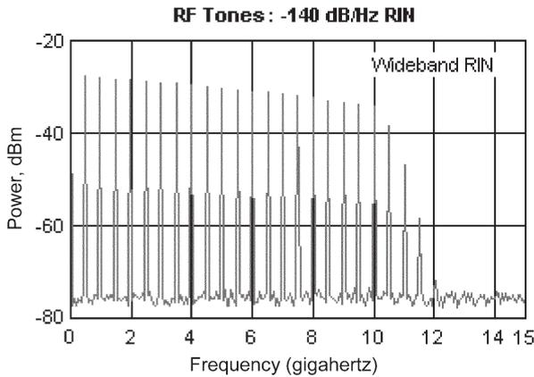
Fig. 12. RF spectrum for  $-140$  dB/Hz laser RIN (unfiltered).
