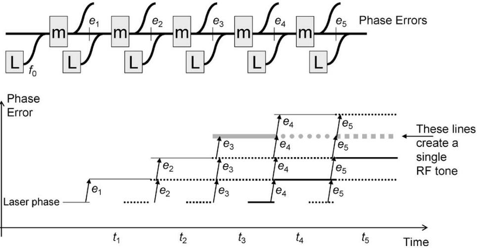
Fig. 18. Unwound ring model with phase errors along the path. If the phase errors are constant ( $e_1 = e_2 = e_3 = \dots$ ), then a particular optical line will have a constant phase with no discontinuities, as shown in the graph.
