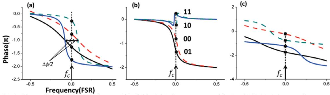
Fig. 2 : Three typical example of solution sets of  $(s_3,s_3)$   $(s_3,s_4)$   $(s_1,s_2)$   $c$  parameter combinations (a) (b) (c). 4 phases can be generated in each case at carrier frequency  $f_c$ .
