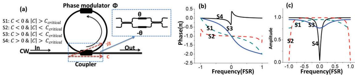
Fig.1 (a) A schematic of ring resonator modulator; (b) Typical phase response shapes of four status; (c) Corresponding amplitude responses.
