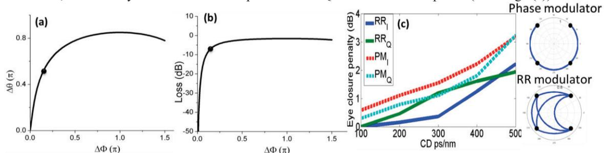
Fig.3. (a) Phase shift required for the RR modulator ( $\Delta\theta=|\theta_1-\theta_2|$  and  $\Delta\phi=|\phi_1-\phi_2|$ ); (b) Transmission loss against  $\Delta\phi$ ; (c) eye closure penalty vs. chromatic dispersion for RR modulator and phase modulator. Inset: transition path of RR and phase modulator. Markers on (a) and (b) show the operating point for the simulation shown in (c).
