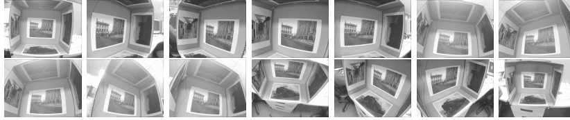
Figure 3. Box dataset: photographs taken of a test rig (consisting of photographs pasted to the inside of a cuboid) with strong changes of perspective, changes in scale and large amounts of radial distortion. This tests the corner detectors on planar textures.
