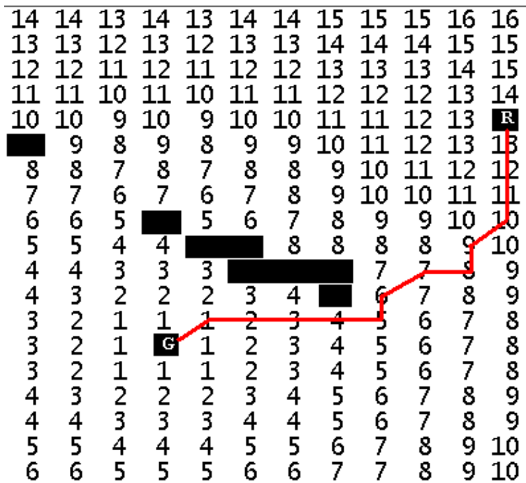
Figure 1: Distance transform and the path formed between a robot and its goal point.
