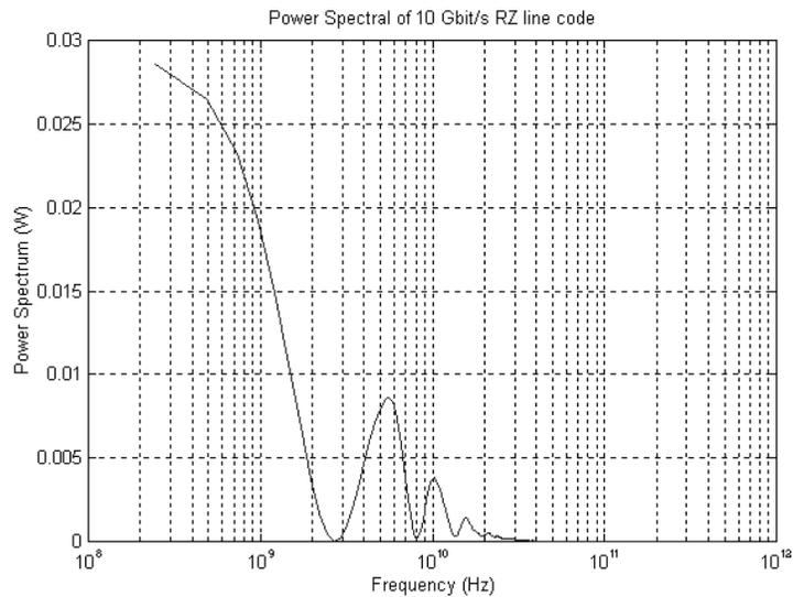
**Figure 2.7** Bandwidth display of RZ line code at 10 Gbit/s
