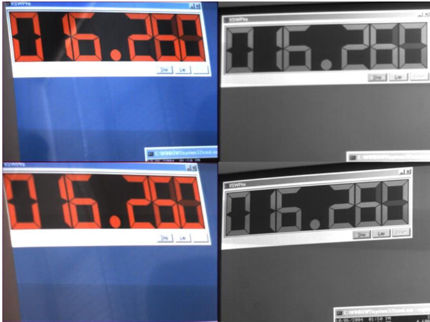
Figure 7.7: Stopwatch images from all 4 cameras for a frame near the start of capture. The top-left and bottom-left colour cameras are both located on the same FireWire bus on one host PC. The top-right and bottom-right mono cameras are both located on the same FireWire bus on a different host PC.
