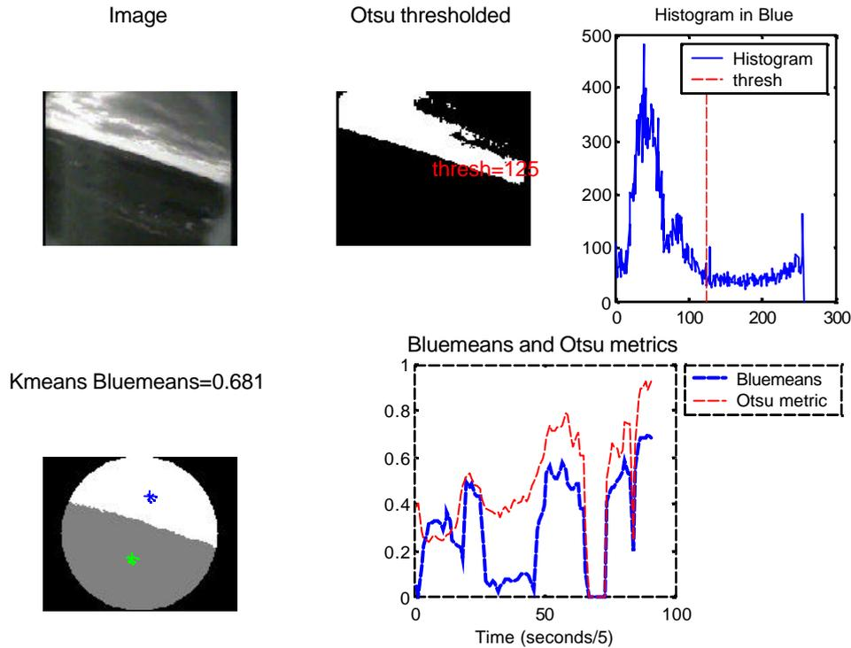
Fig. 10 K-means classifier compared to Otsu's, showing better result.
