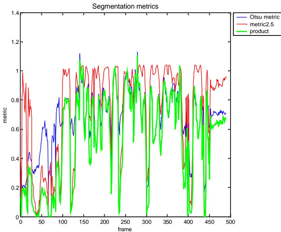
*Fig. 7 Metric2.5 applied to Otsu thresholded video*
