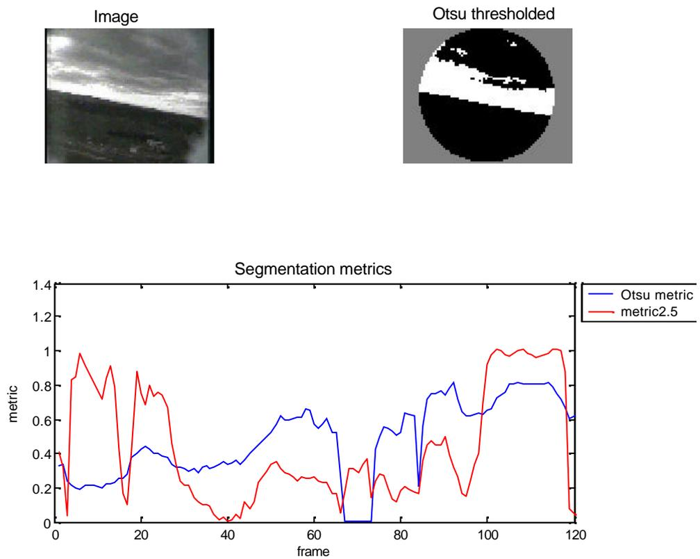
Fig. 9 Example where metric2.5 has low value and Otsu metric has high
