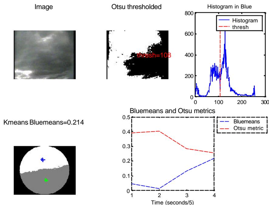
Fig. 11 K-means clustering showing a poor classification result
