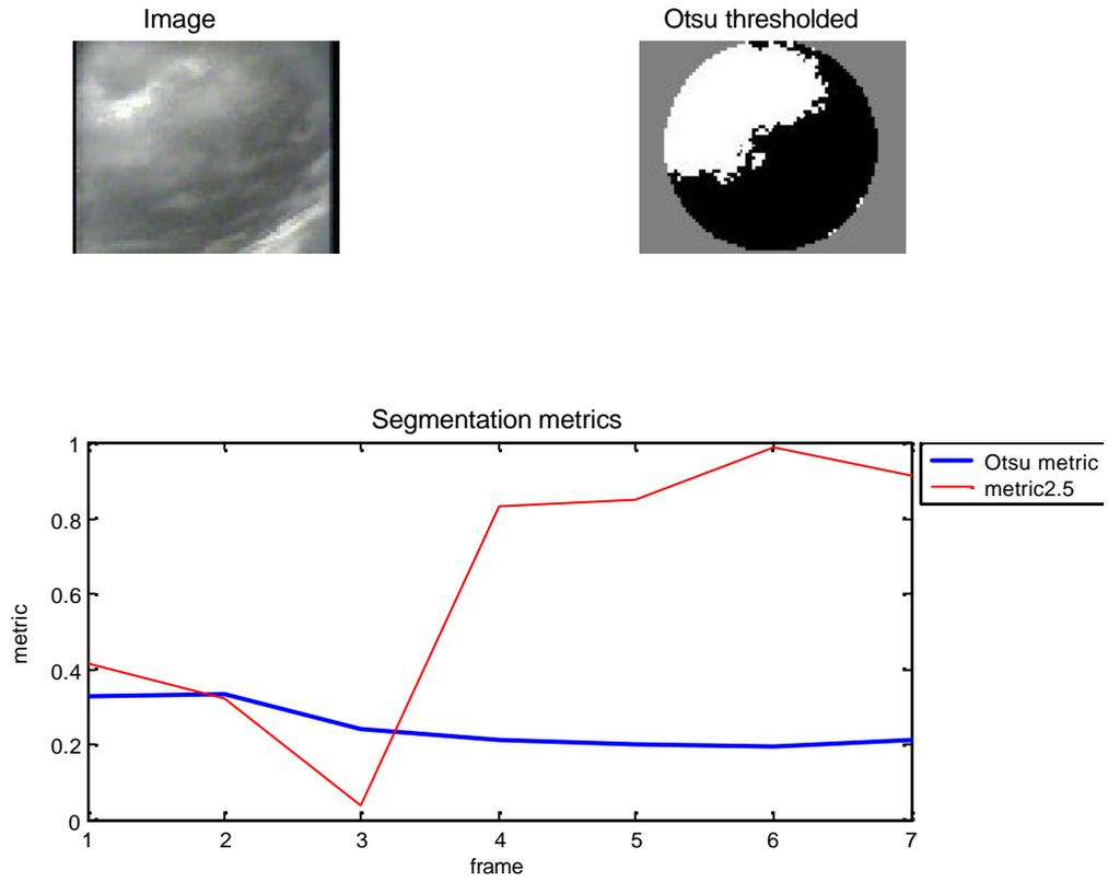
Fig. 8 Metric2.5 showing high value for misclassified frame.
