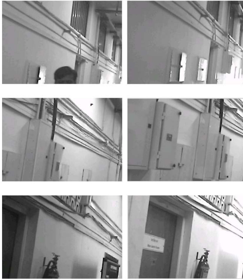
Figure 11 Left column shows images from webcam during localization and right column shows best matched image in database
