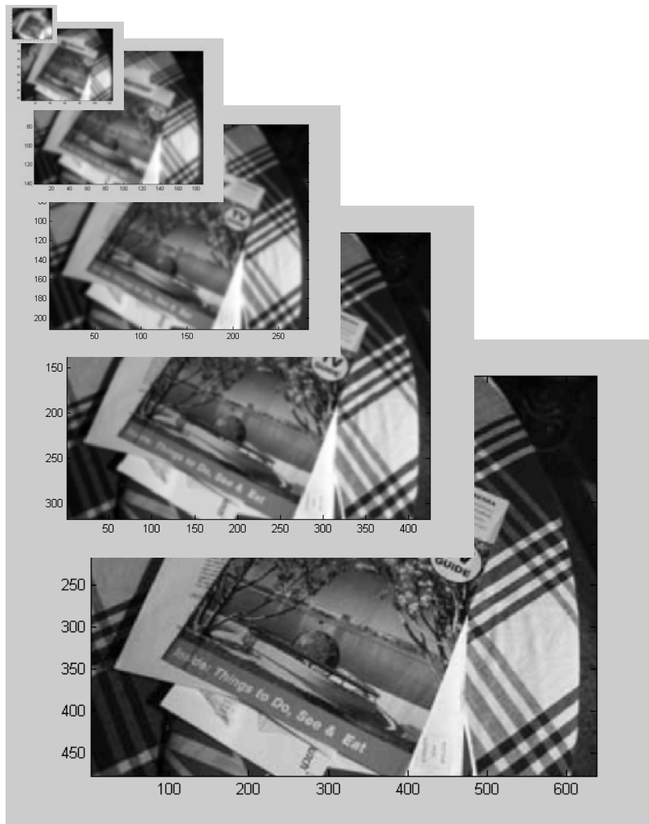
Figure 2 A Gaussian pyramid constructed by successively Gaussian blurring and downsampling an image. Lower layers of the pyramid (toward the bottom of the figure) reveal finer details, like the writing on the TV Guide, but higher layers of the pyramid reveal only coarser details like the outline of the TV Guide.
