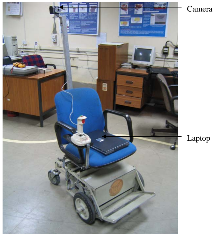
Figure 1 Motorized wheelchair equipped with camera and laptop acts as the mobile platform for testing the localization algorithm
