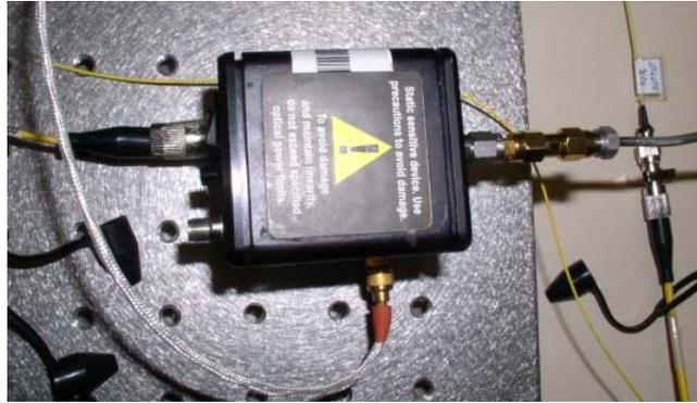
*Figure 11: 12GHz IR Photo Receiver*
