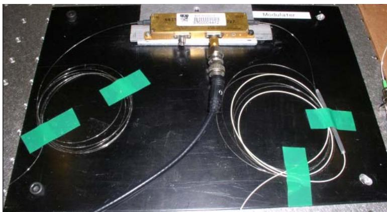
Figure 14: Mach-Zehnder Interferometer Modulator
