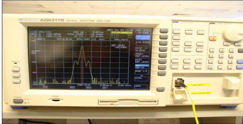
**Figure 4: Optical Spectrum Analyzer**
