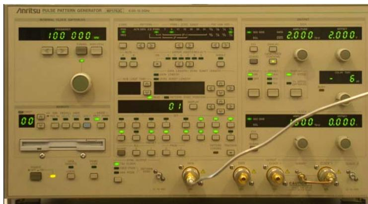
**Figure 7: Pulse Pattern Generator**
