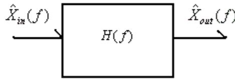
*Figure 17: Block diagram of the linear fiber model, a low pass optical filter.*
