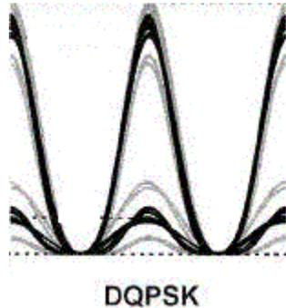
**Figure 21:** The darker eye traces in this eye diagram are the expected traces, the light traces are after phase offset noise due to the instability of the "phase tuning" heater.
