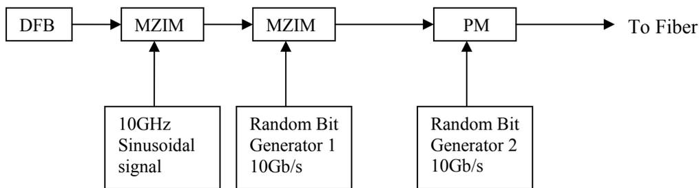
*Figure 9: Schematic of a channel implementing RZ-DQPSK modulation.*
