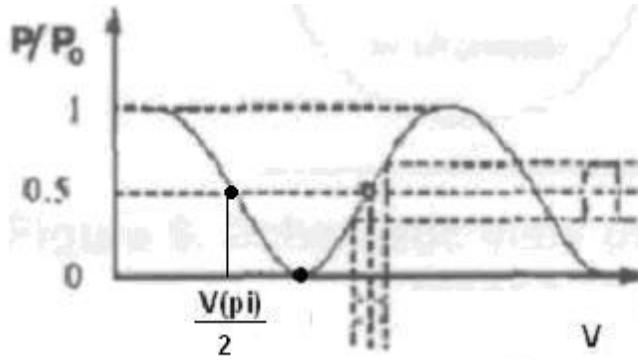
Figure 13: Biasing points of MZIM used for RZ pulse carving (shaping), carrier suppression if biased at the minimum transmission point ( $V_{pi}$ ) or maximum transmission point if carving not required.
