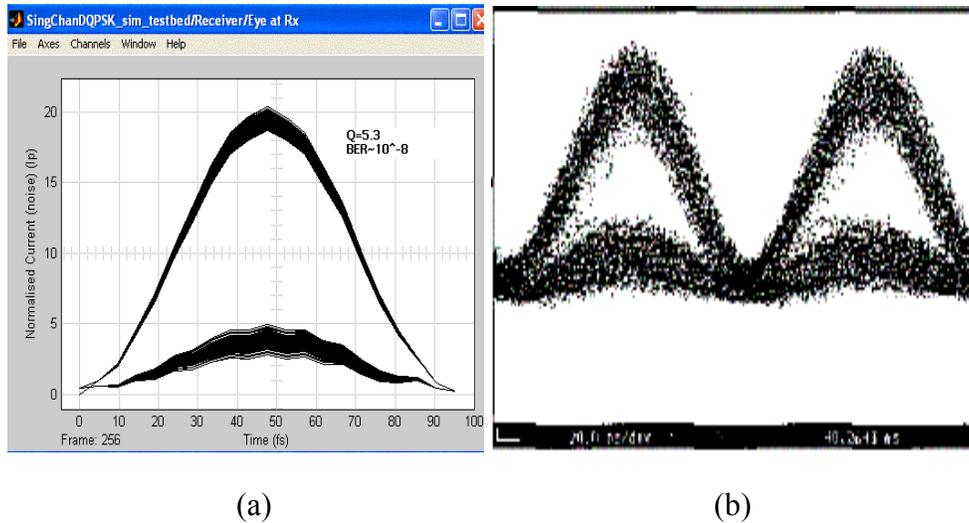
**Figure 34:** Single-ended simulated eye diagram (a), Eye diagram source obtained via experimental investigation from literature search using a similar transmitter configuration to the simulator (b)[18].
