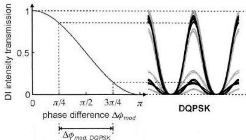
**Figure 5:** The phase to intensity characteristic of the MZDI and the expected eye diagram generated at the output of the MZDI based on the phase difference between the two arms, the lighter eye pattern is due to phase offset,  $\delta\phi_{DI}$ , from heater
