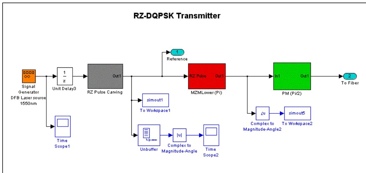
Figure 10: Simulink model of Figure 9, the unit delay block samples the continuous Signal generator waveform at Nyquist rate.
