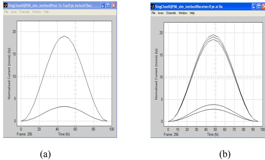
*Figure 29: Electrical current eye diagram generated before fiber (a) and at Rx(b). Using SMF link, without DCF, no PD and amplifier noises and no MZDI phase offset. This eye effectively shows the dispersion effects of SMF alone on the eye closure and thence on BER. The phase to intensity converted by the receiver no longer has two distinct levels as on the left (a).*
