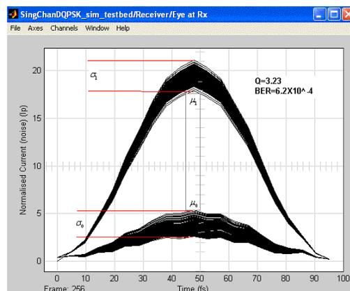
**Figure 30:** Electrical current eye diagram generated at Rx with SMF link, No DCF inserted with PD and amp noise added.
