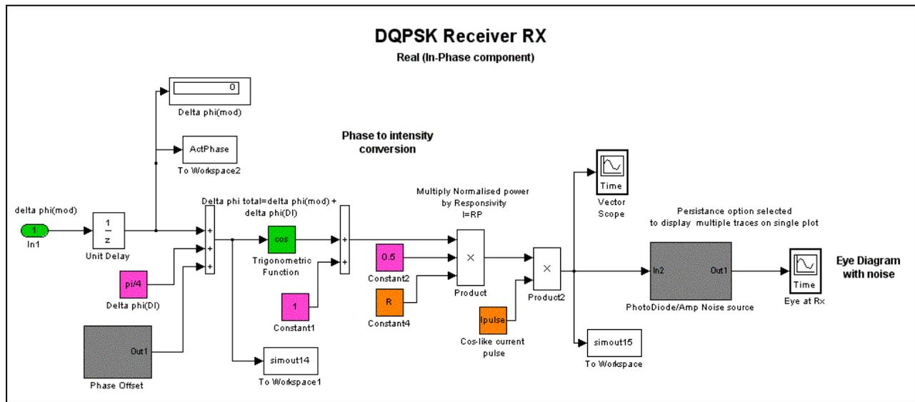
*Figure 20: Receiver model including noise sources*
