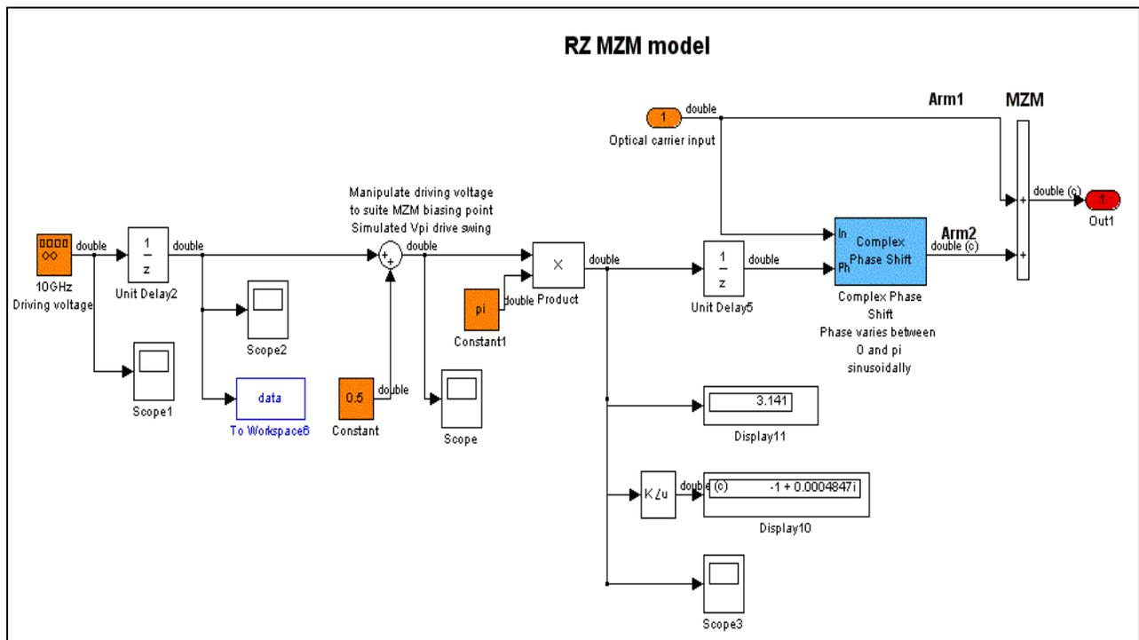
Figure 14: The Simulink RZ MZIM model
