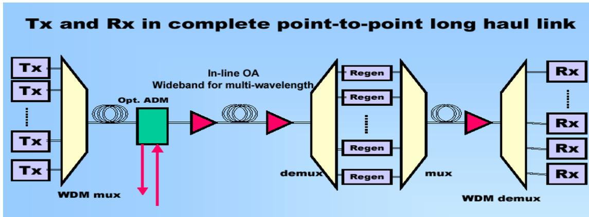
*Figure 1: Typical architecture of DWDM transmission system*
