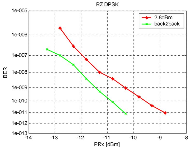
Figure 62 Transmission over 50 km SSMF: BER versus Rx sensitivity with total launched power as a parameter. Modulation format: RZ-DPSK
