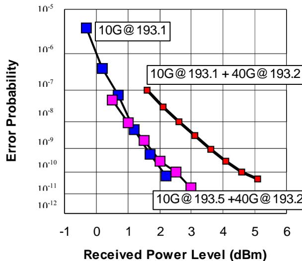
The set up of the transmission system with 320km SSMF and dispersion compensating module with 2 100GHz AWG's as muxes and Rx filter to measure the impact of adjacent CS-RZ DPSK 40G channel on 10G NRZ-ASK performance. No significant impact noted when 40G channel, adjacent or non-adjacent, is switched on. (Note: demo only as 40G channel would not actually perform well through such a narrow filtering arrangement).
