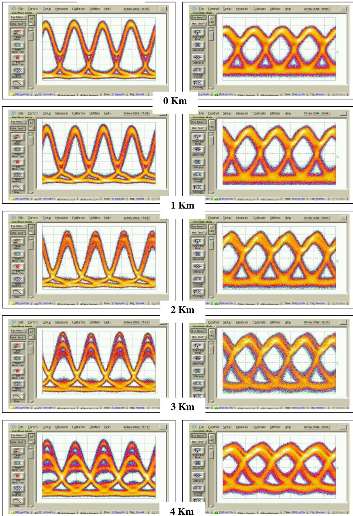
Figure 13 Samples of eye diagrams of phase difference NRZ-DPSK and CSRZ ASK modulation formats – SSMF length is a parameter.
