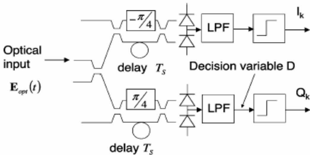
Figure 6 Balanced receiver structure for phase difference modulation format. Note it is a parallel structure of two DPSK balanced receiver with additional phase shifting of  $\pi/4$
