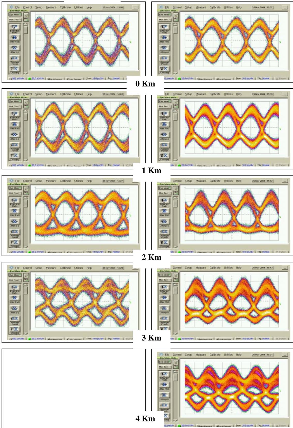
Figure 14 Samples of eye diagrams of phase difference modulation formats – SMF length is a parameter.
