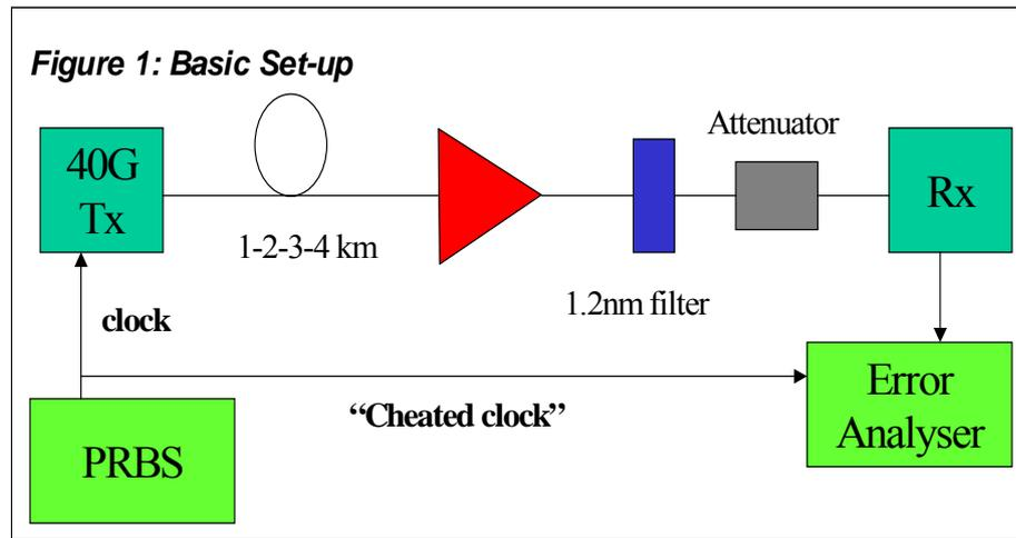
Figure 7 Schematic diagram of the experimental set-up for measurement of the dispersion tolerance of modulation formats.
