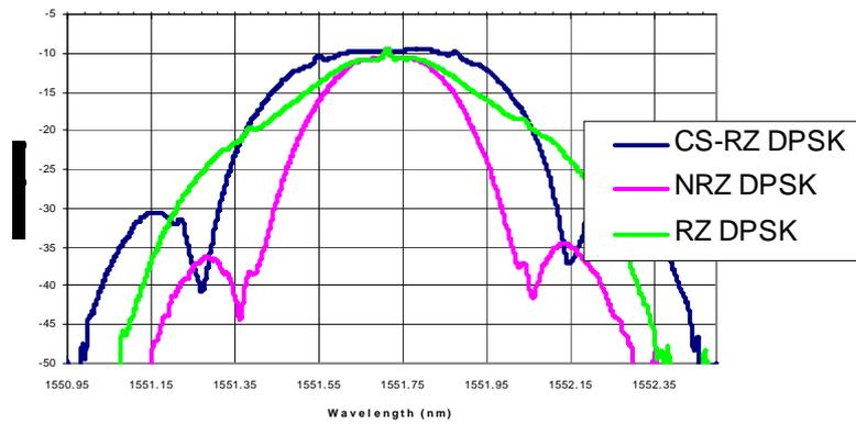
Figure 9 Optical spectra of CS-RZ DPSK, NRZ DPSK and RZ DPSK – base rate 40 G
