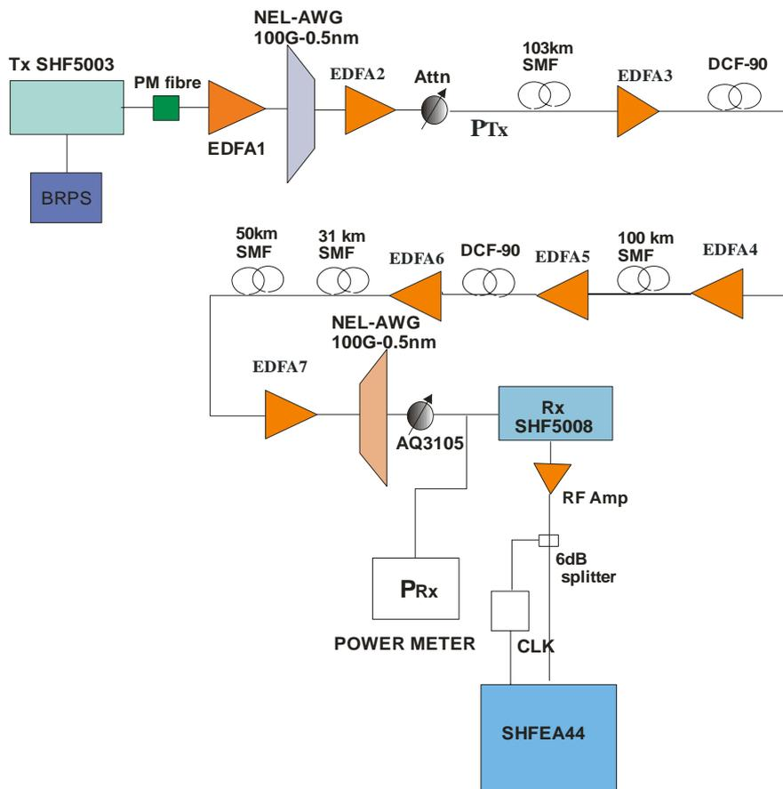
Figure 63 - Experiment setup: CSRZ DPSK 230km transmission, 234km SMF + DCF for 230km
