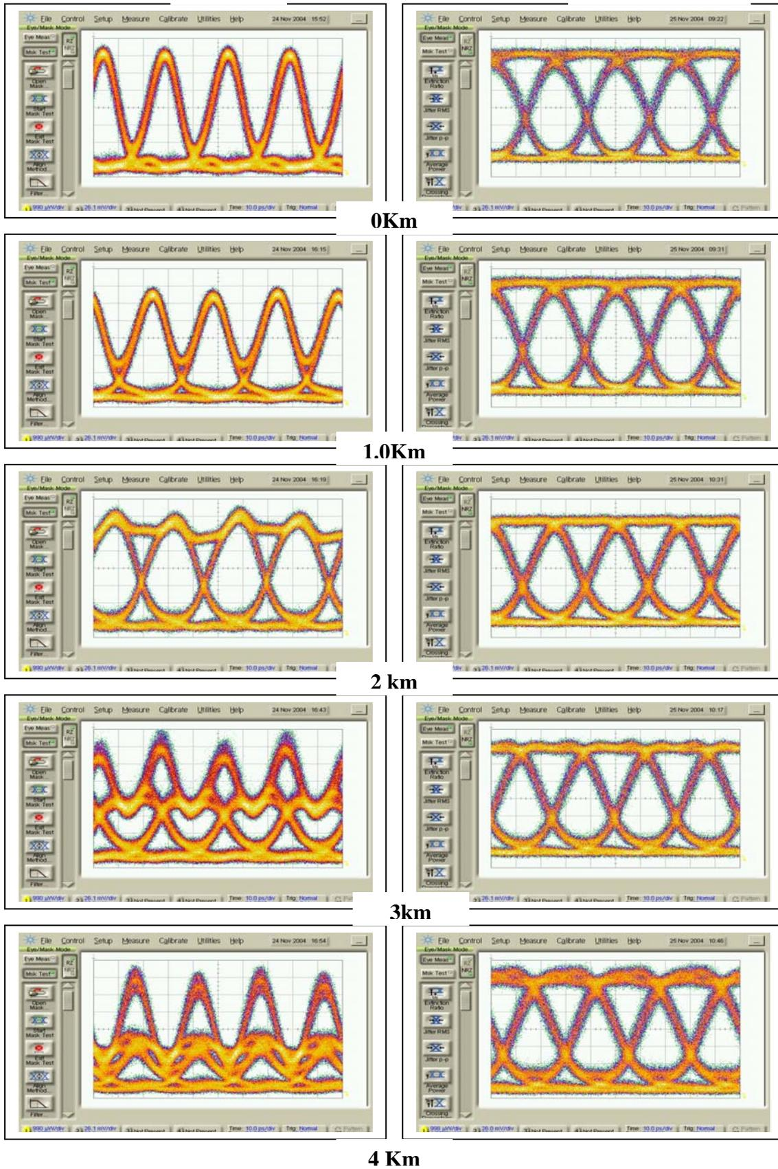
Figure 12 Samples of eye diagrams of ASK modulation formats – SSMF length is a parameter.
