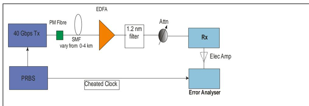
Figure 42 Experimental set up to measure the dispersion tolerance of different modulation formats.
