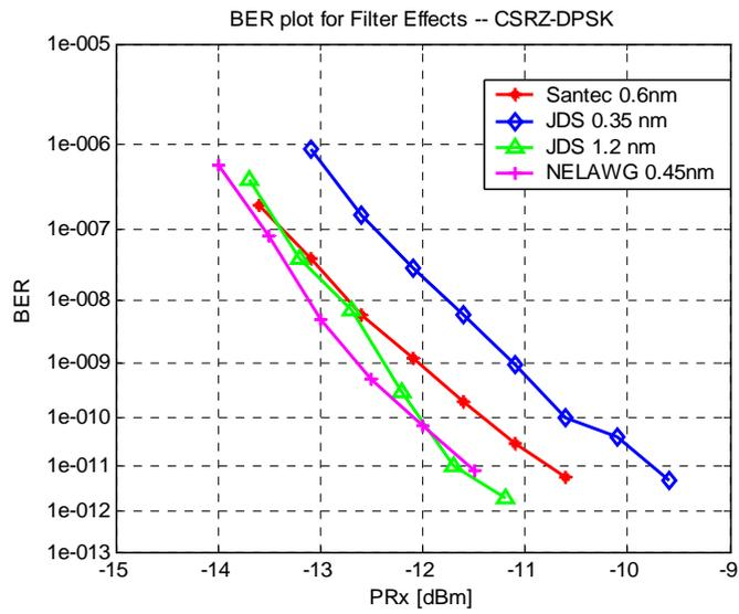
Figure 67 Optical filtering effects: BER versus Rx sensitivity format CS\_RZ DPSK
