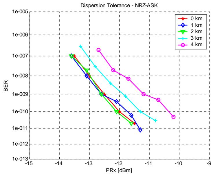
Figure 45 BER as a function of receiver sensitivity with SSMF length as a parameter. Modulation format: RZ-ASK.
