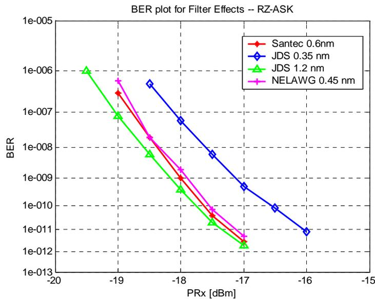
Figure 71 BER versus Rx sensitivity format RZ ASK
