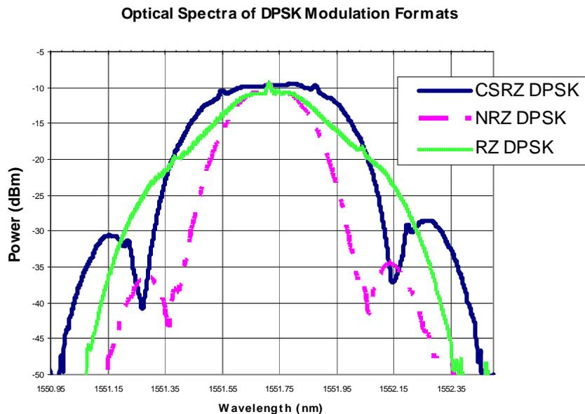
Figure 35 Optical spectra modulation formats phase shift keying of various formats
