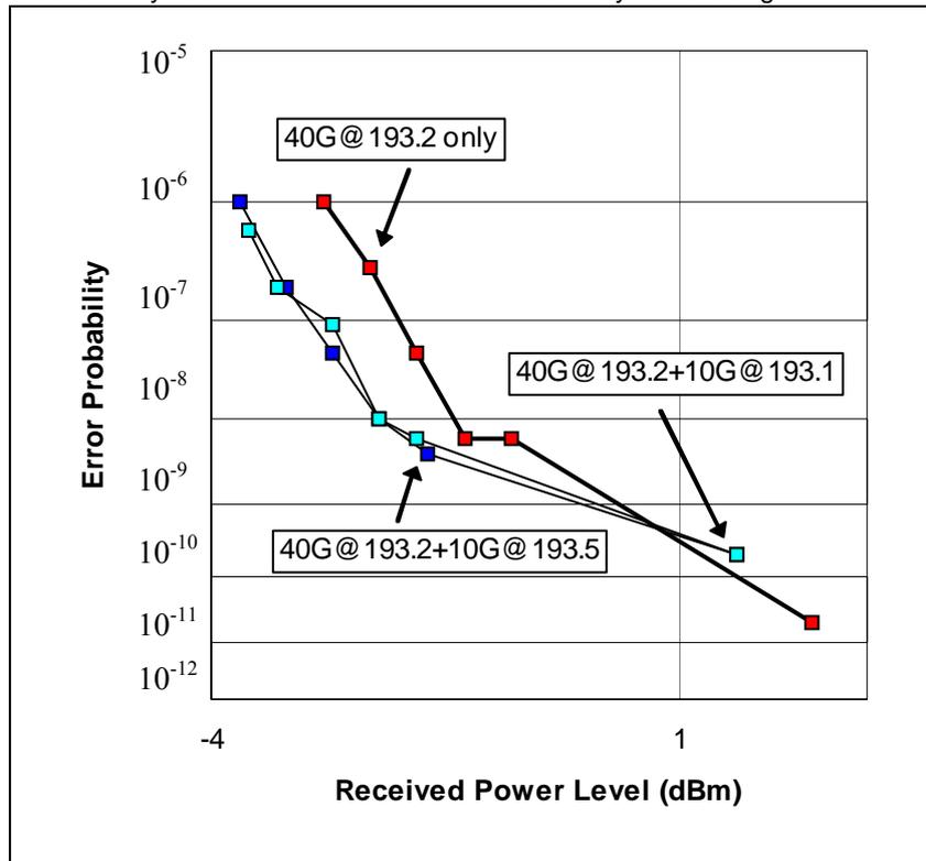
Figure 41 Impact on 40 G with 10 G channel transmission 320 km transmission: Probability of error versus receiver sensitivity (dBm)- effects of 40 G (CS\_RZ DPSK) with 10G (NRZ-ASK) channel simultaneously transmitted for NRZ ASK and CS-RZ DPSK formats – blue dots for 1.2 nm thin film filter and dots for two 0.5 nm AWG filter (demux with 200 GHz spacing)
