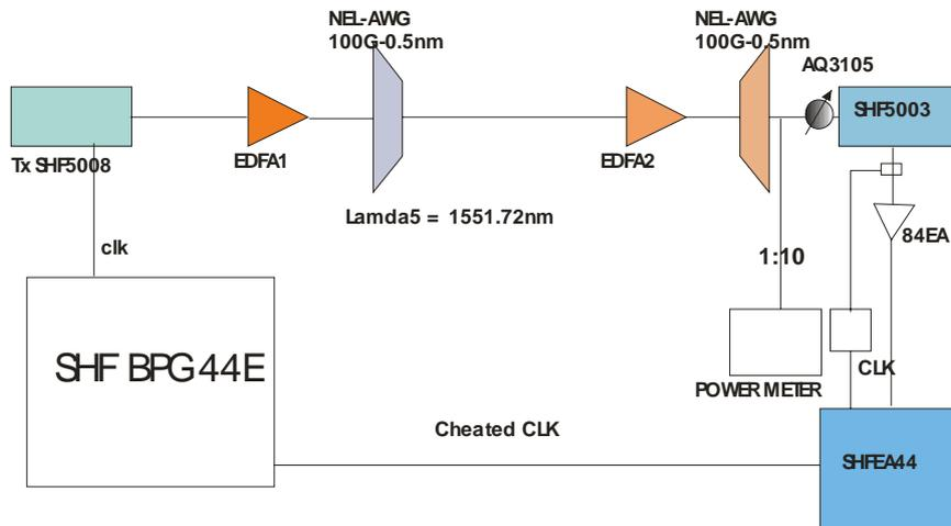
Figure 29 Experimental set-up to measure the optical filtering on modulation formats–Optical filters:ONE FILTER NEL – AWG ONLY.
