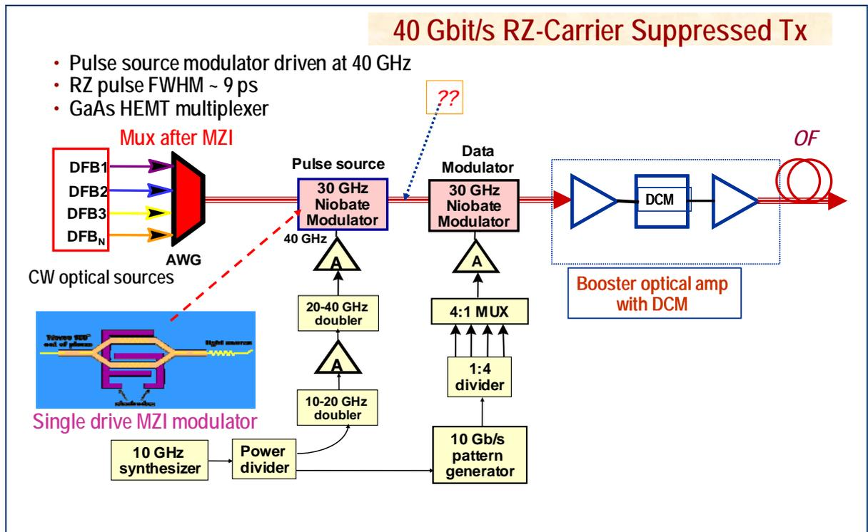
Figure 3 Structure of external modulation for generation of advanced modulation format lightwave signals.
