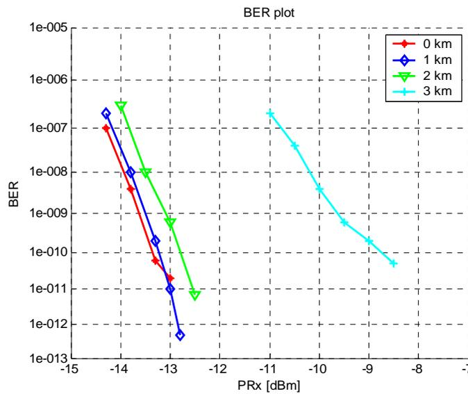
Figure 43 BER as a function of receiver sensitivity with SSMF length as a parameter. Modulation format: RZ - ASK.
