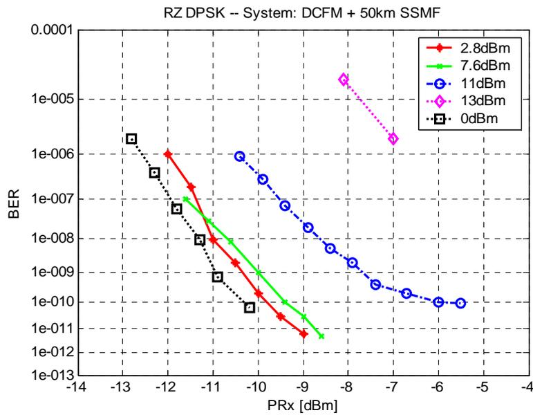
Figure 57 transmission over 50 km SSMF: BER versus Rx sensitivity with total launched power as a parameter. Modulation format: RZ-DPSK
