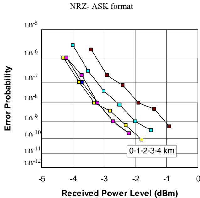
Figure 15 BER versus receiver sensitivity (-10dB) for NRZ format transmission back to back (0km) and 1-4 km of SSMF.
