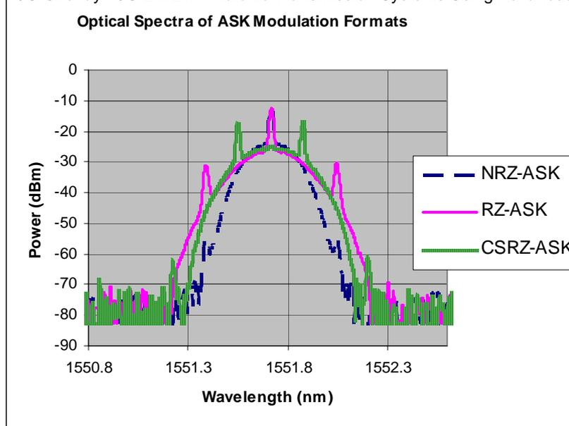
Figure 34 Optical spectra modulation formats amplitude shift keying of various formats
