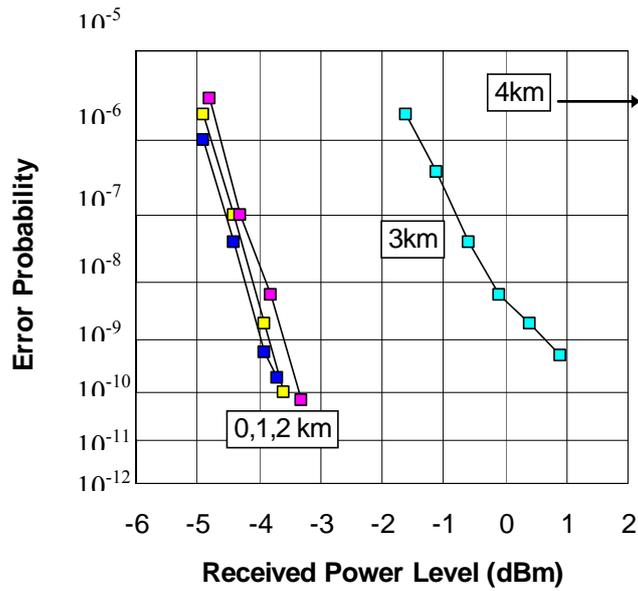
Figure 17 BER versus Rx sensitivity (-10dB) – modulation format RZ ASK
