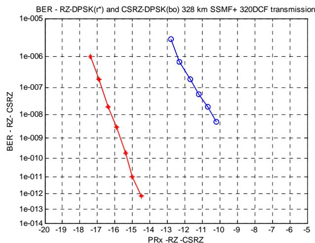
Figure 28 Transmission system: dispersion management 328 kmSSMF + DCM320 compensating fibers. Note: MUX is NEL AWG 0.5 nm 100 GHz Spacing and DEMUX is 1.2 nm OF (thin film structure) (see red curve) – blue is for NEL-AWG+NEL-AWG (100 GHz spacing and 0.5 nm BW) as MUX and DEMUX
