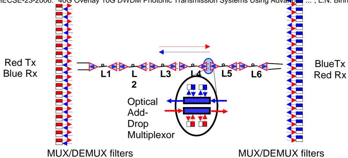
Figure 1 Schematic diagram of a long haul photonic transmission system.  $L$  = length of the transmission fiber, dispersion compensating fibers (DCF) hidden in the optical amplifiers denoted. Two optical amplifiers are used one as optical pre-amp and the other booster amplifiers. Photonic muxes and demuxes are array waveguide (AWG)
