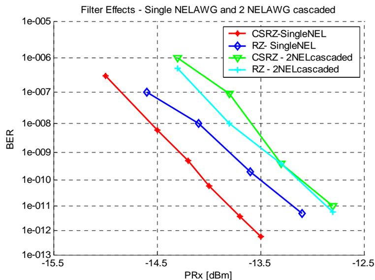
Figure 50 Effects of filtering - BER as a function of receiver sensitivity with modulation formats as a parameter: CSRZ-ASK, RZ-ASK and CSRZ-ASK
