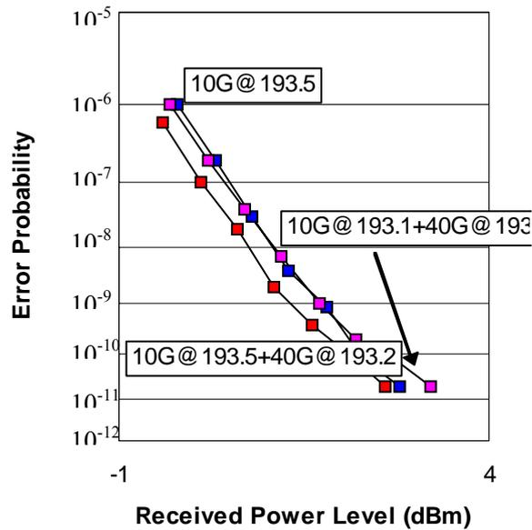
Figure 40 320 km transmission 40 G impact on 10G channel: Probability of error versus receiver sensitivity (dBm)- effects of 40 G (CS\_RZ DPSK) with 10G (NRZ-ASK) channel simultaneously transmitted for NRZ ASK and CS-RZ DPSK formats – blue dots for 1.2 nm thin film filter and dots for 0.5 nm AWG filter (demux with 100 GHz spacing)
