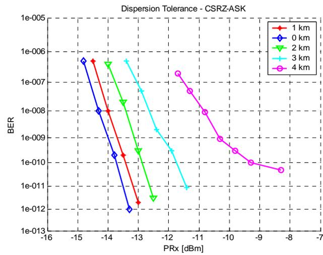
Figure 44 BER as a function of receiver sensitivity with SSMF length as a parameter. Modulation format: carrier-suppressed RZ.
