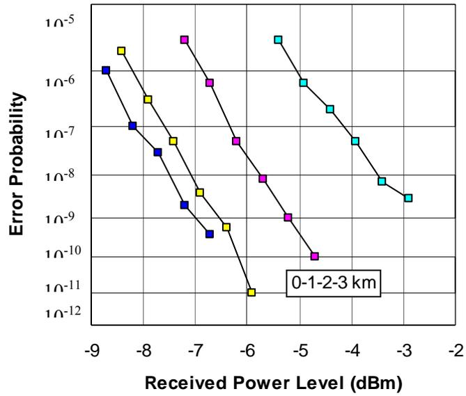
Figure 20 BER versus receiver sensitivity (-10dB) power obtained for CS-RZ – DPSK format with back-to-back (0km) and 1-4 m SSMF. . Note the ~3-4dB improvement of the RZ type DPSK's over ASK formats.
