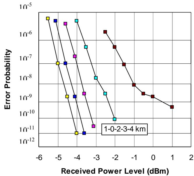
Figure 18 BER versus Rx sensitivity (-10dB) – modulation format CS\_RZ ASK. Yellow dots are for back-to-back.
