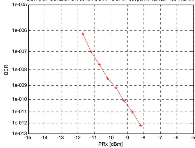
Figure 23: Receiver sensitivity of the CSRZ-DPSK modulation format. Transmission distance= 50 km SSMF + Sumitomo DCFM (-850 ps/nm @ 1550nm) – source wavelength lamda 5 = 1551.72 nm CSRZ-DPSK transmission after 50 km SSMF and DCFM (-850 ps/nm at 1550 nm).
