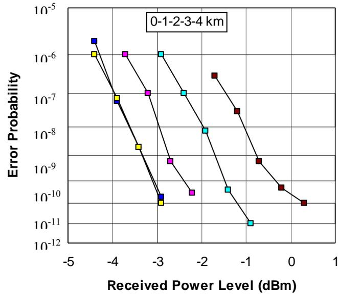
Figure 16 BER versus receiver power obtained for NRZ – DPSK format with back-to-back (0km) and 1-4 m SSMF.
