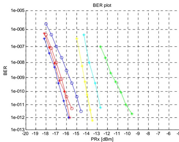
Figure 32 BER versus received optical power (at the power meter – 1;10 coupler before Rx). Legends: “blue” CSRZ-DPSK (one NELAWG); “red” – RZ DPSK(one NELAWG); “green” NRZ ASK(one NELAWG); “yellow” – CSRZ- ASK (one NELAWG); “c” RZ-ASK(one NELAWG); Note: only one optical filter NEL AWG is used; “Red o” CSRZ DPSK TWO AWGs used; “blue o” RZ-DPSK TWO AWGs used
