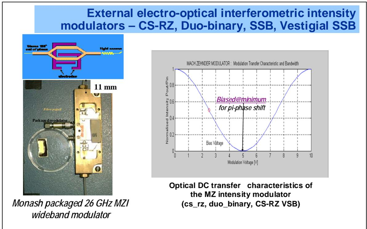
Figure 4 MZIM structure, packaged device and operating characteristics – the transfer curve.
