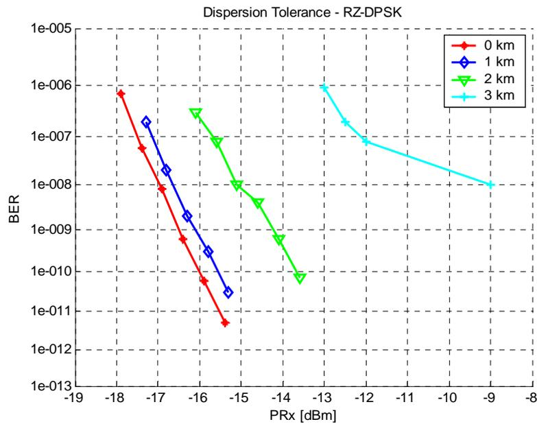
Figure 46 BER as a function of receiver sensitivity with SSMF length as a parameter. Modulation format: RZ-DPSK.
