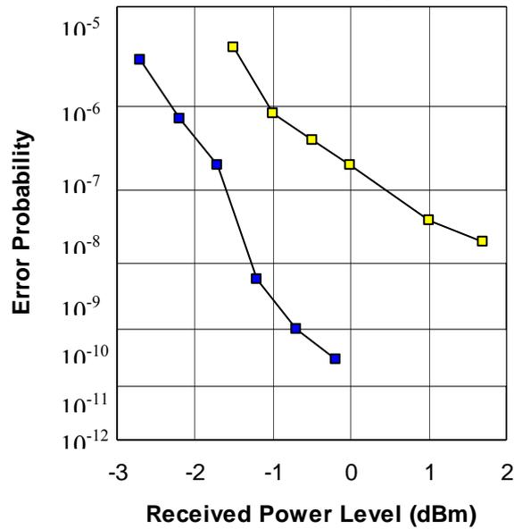
Figure 36 Probability of error versus receiver sensitivity (dBm) for CS-RZ format – blue dots for 1.2 nm thin film filter and yellow dots for 0.5 nm AWG filter (demux with 100 GHz spacing)
