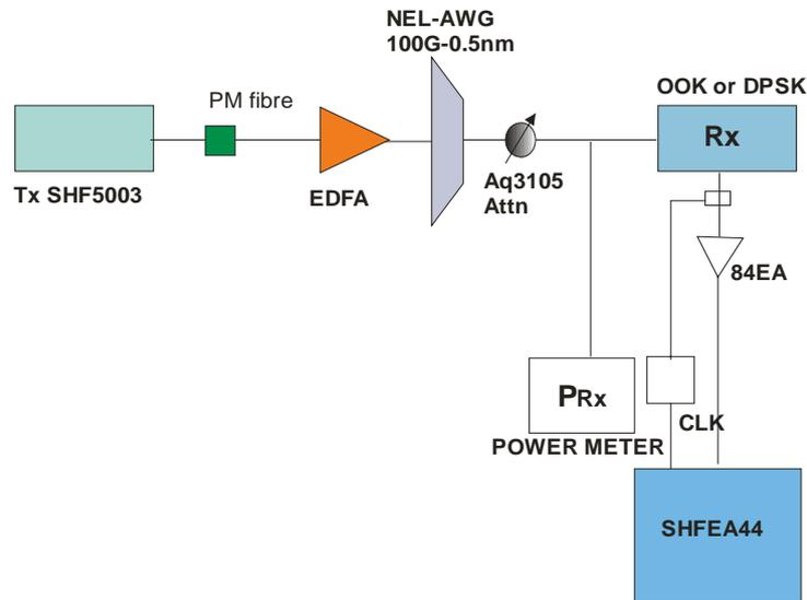
Figure 66 Measurement set-up of BER and Rx sensitivity due to filter effects
