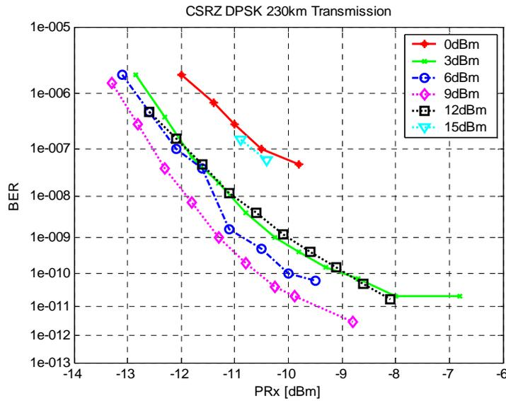
Figure 64 Figure 65 transmission over 234 km SSMF: BER versus Rx sensitivity with total launched power as a parameter. Modulation format: CSRZ-DPSK
