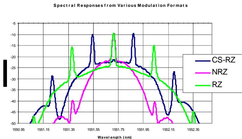
Figure 8 Optical spectra of CS-RZ ASK, NRZ-ASK and RZ-ASK – base rate 40 G
