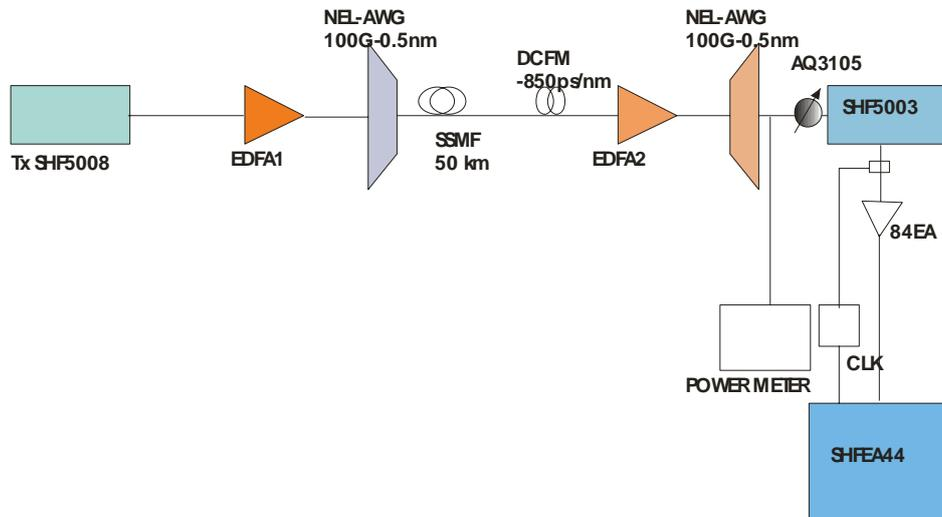
Figure 22 Dispersion managed 50 km SSMF + DCFM transmission system set-up
