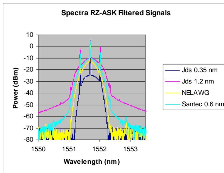
Figure 72 Optical spectra of optically filtered format RZ-ASK
