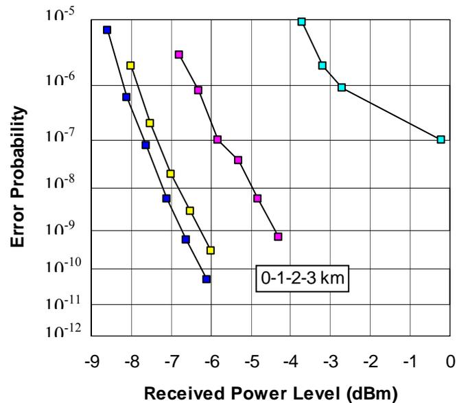
Figure 19 BER versus receiver sensitivity (-10dB) power obtained for RZ – DPSK format with back-to-back (0km) and 1-4 m SSMF.
