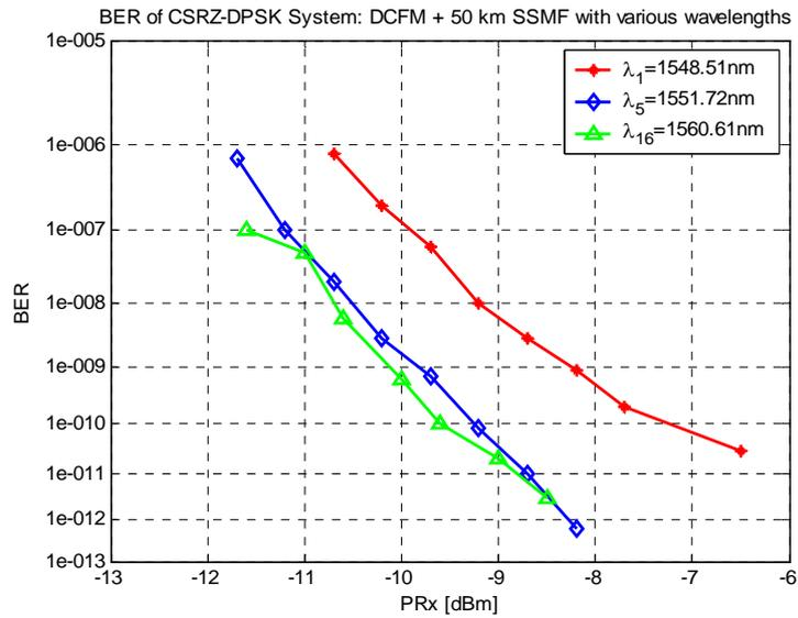
Figure 54 transmission over 50 km SSMF: BER versus Rx sensitivity. Modulation format: CSRZ-DPSK
