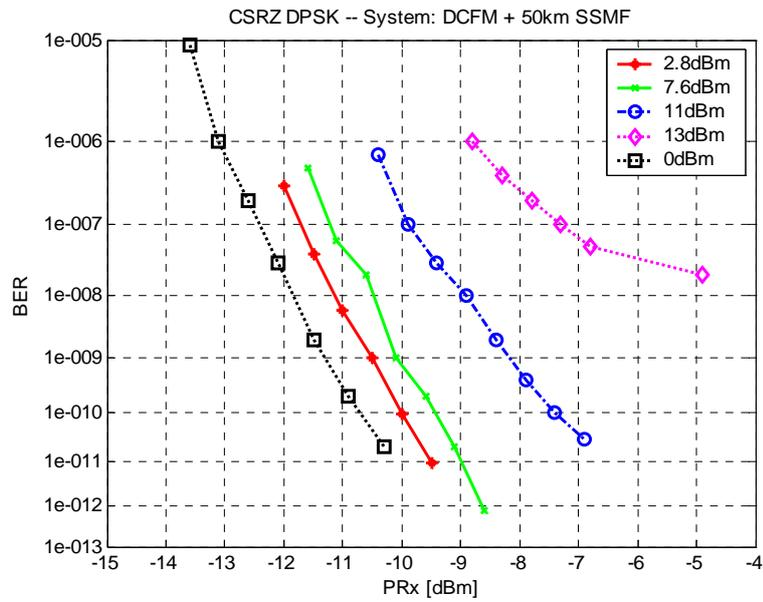
Figure 56 Transmission over 50 km SSMF: BER versus Rx sensitivity with total launched power as a parameter. Modulation format: CSRZ-DPSK.
