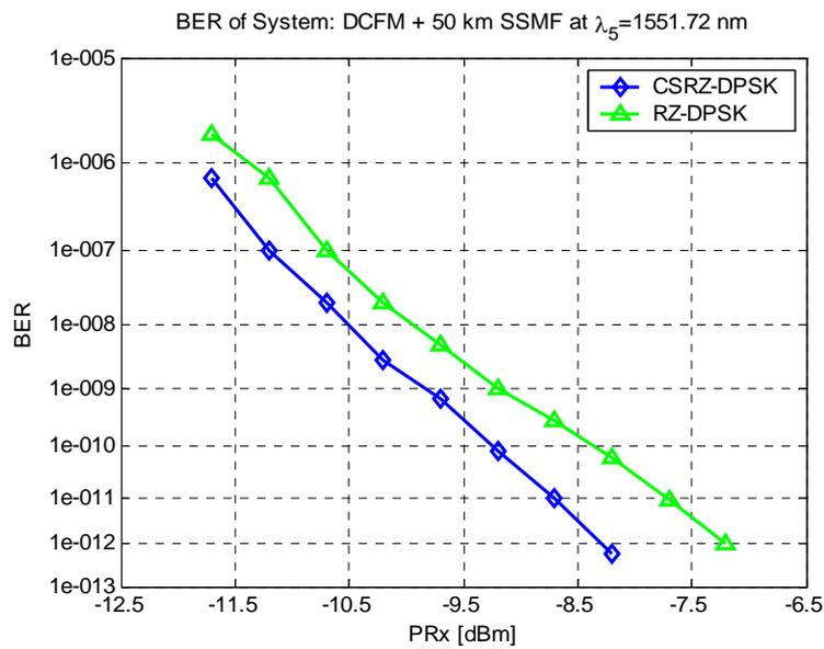
Figure 55 transmission over 50 km SSMF: BER versus Rx sensitivity. Modulation format: CSRZ and RZ- DPSK.
