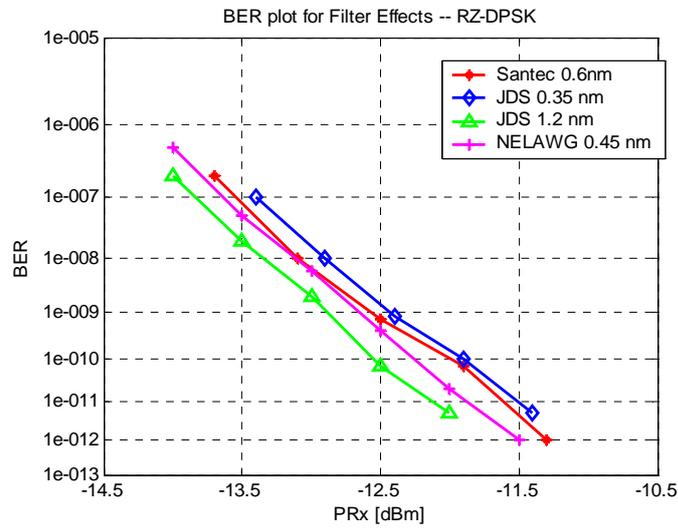
Figure 69 BER versus Rx sensitivity format RZ DPSK
