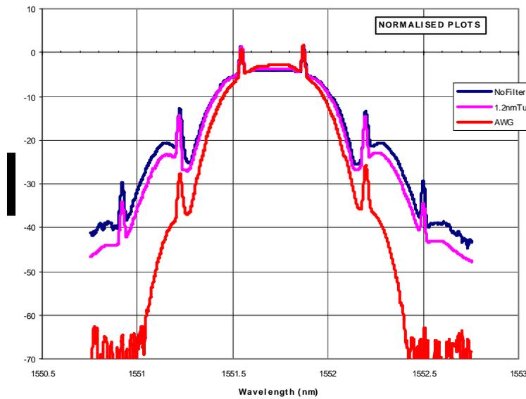
Figure 11 Optical spectra of CS-RZ – base rate 40 G after optical filters thin film and AWG types.
