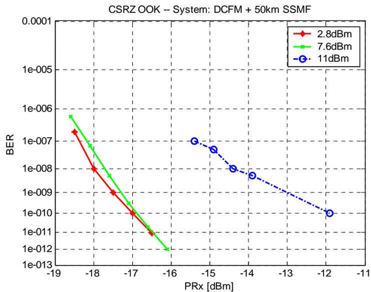
Figure 58 transmission over 50 km SSMF: BER versus Rx sensitivity with total launched power as a parameter. Modulation format: CSRZ-ASK
