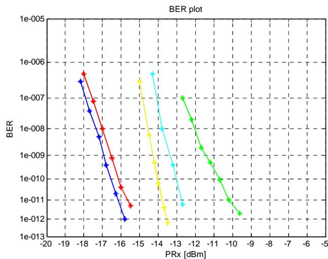
Figure 30 BER versus received optical power (at the power meter – 1;10 coupler before Rx). Note: “blue” CSRZ-DPSK; “red” – RZ DPSK; “green” NRZ ASK; “yellow” – CSRZ-ASK; “c” RZ-ASK; Note’ bien: only one optical filter NEL AWG is used
