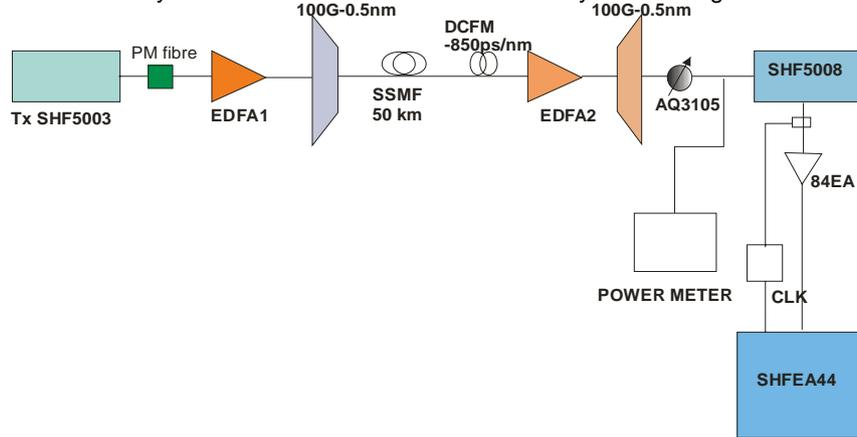
Figure 33 50 Km SSMF transmission experimental set-up
