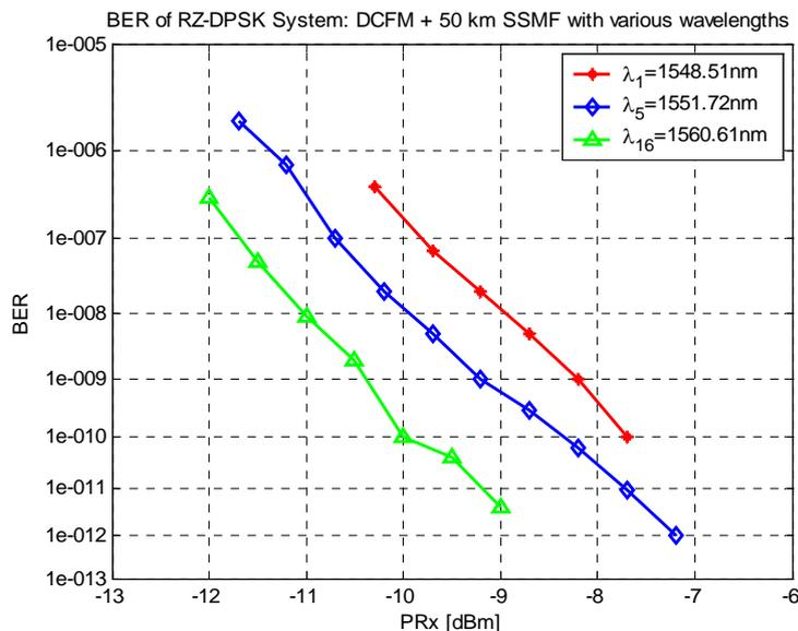
Figure 53 transmission over 50 km SSMF: BER versus Rx sensitivity. Modulation format: RZ-DPSK.
