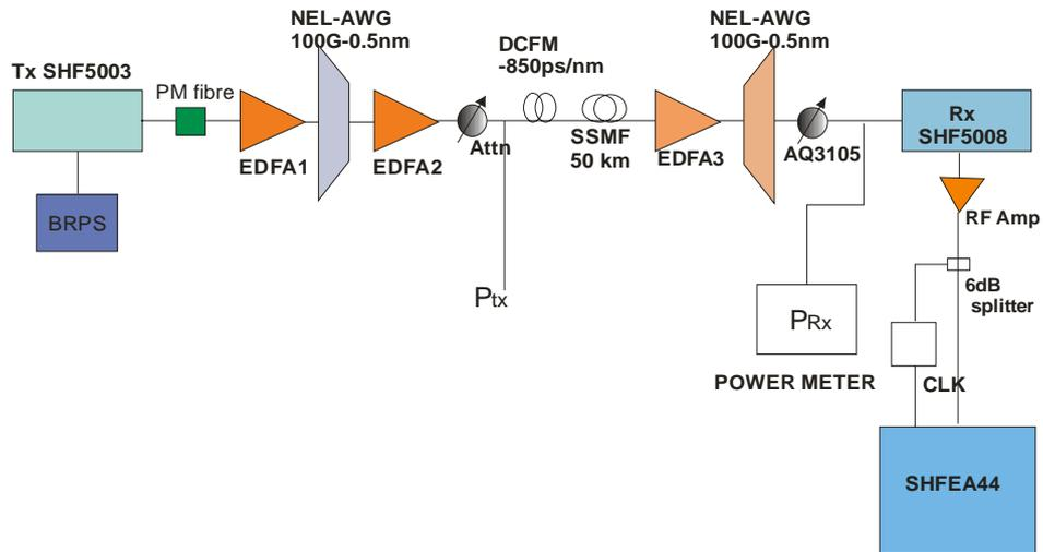
Figure 52 50 km DCF + SMF Transmission system set-up
