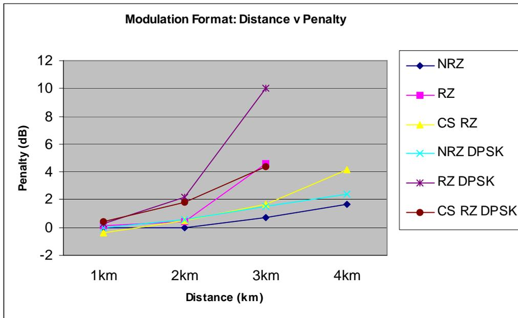
Figure 21 Power penalty as a function of the transmission distance for various modulation formats
