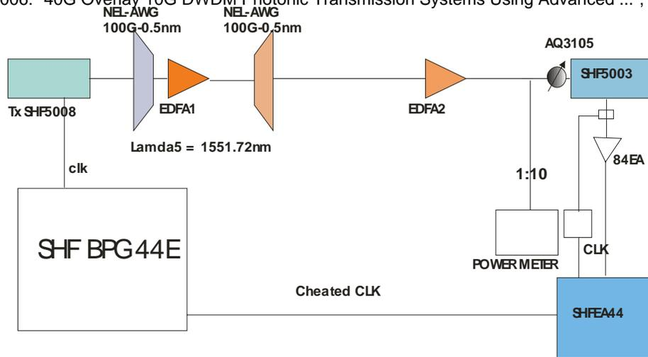
Figure 31 Experimental set up –OPTICAL FILTER EFFECTS (TWO FILTERS NEL – AWG +EDFA +NEL- AWG +EDFA) ON MODULATION FORMAT. Note: only CSRZ-DPSK and RZ-DPSK gives recorded BER, EDFA1 = 176 mW pump power – saturation mode; EDFA2 = 132 mW pump power – saturation mode
