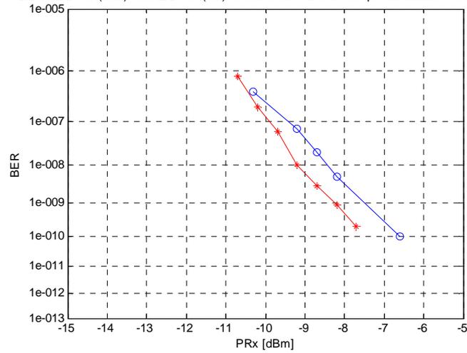
Figure 25: RZ-DPSK (blue) and CSRZ-DPSK (red) modulation format transmission distance= 50 km SSMF + Sumitomo DCFM (-850 ps/nm @ 1550nm) – source wavelength ( $\lambda_1$ )= 1548.51 nm. MUX and DEMUX NEL-AWG circulant filter and spacing demultiplexing.
