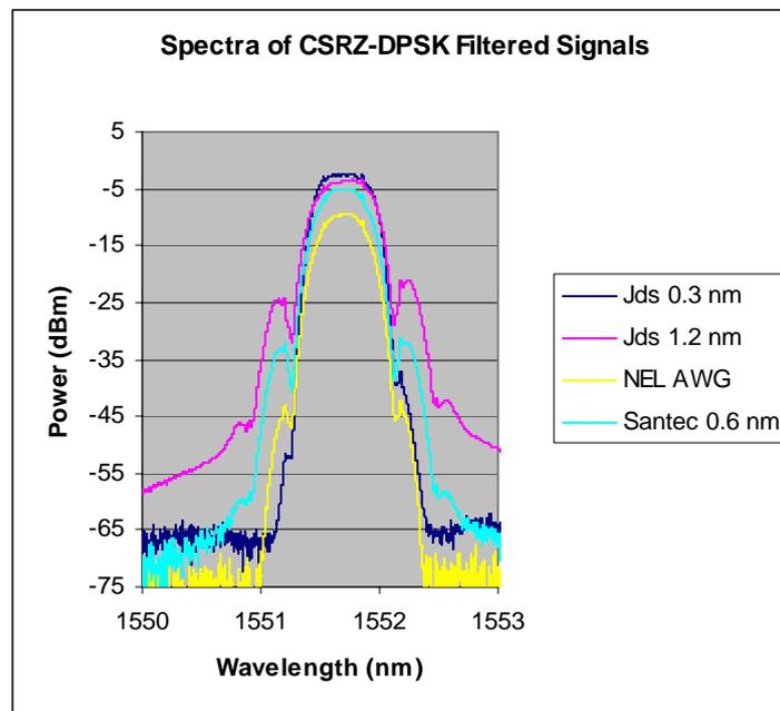
Figure 68 Optical Spectra of filtered lightwave signals
