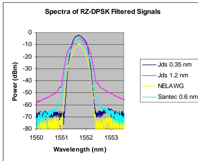
Figure 70 Optical Spectra of filtered lightwave signals- format RZ-DPSK
