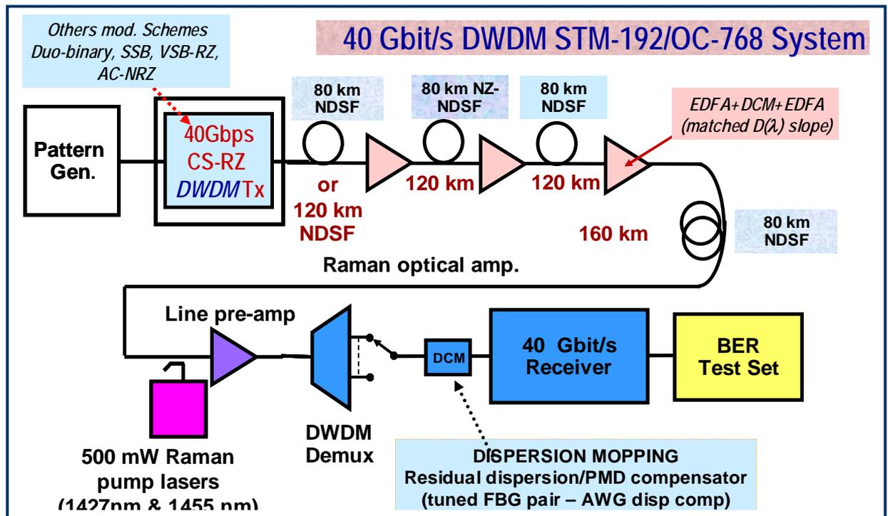
Figure 2 Schematic diagram of a 40G DWDM photonic communication system employing advanced modulation formats.
