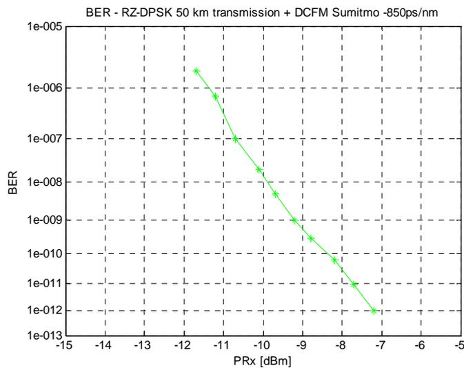
Figure 24 Optical transmission over 50 km of SSMF + DCFM (total dispersion -850 ps/nm); Modulation format = RZ -DPSK, Eye diagram captured at -10.7 dBm at the power meter (1:10 FC port). Note: full clock recovery used for sampling the EA 44E. Centre wavelength (lamda 5) = 1551.72 nm.
