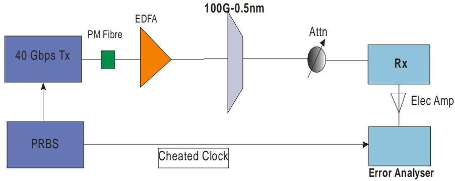
Figure 48 Experimental set up to measure the optical filtering effects on different modulation formats
