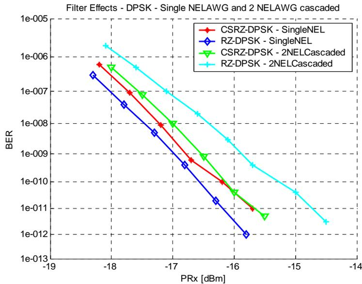
Figure 51 Effects of filtering - BER as a function of receiver sensitivity with modulation format of phase difference: RZ, NRZ and CSRZ.
