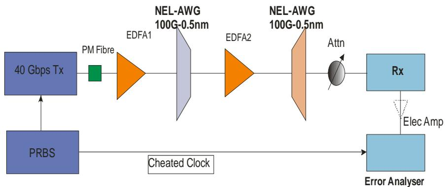
Figure 49 Experimental set up to measure the optical filtering effects on different modulation formats using two filters.
