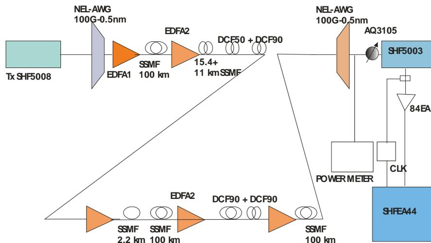
Figure 27 Optically amplified dispersion managed transmission: 328 KM SSMF + 320 DCF transmission with CSRZ-DPSK and RZ – DPSK formats.
