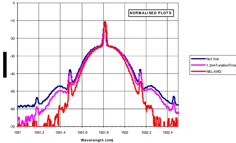
Figure 10 Optical spectra of NRZ-ASK base rate 40 G after the optical filters – thin film 1.2 nm and NEL AWG 0.5 nm passband and no filter.- minimum effect on the spectrum.
