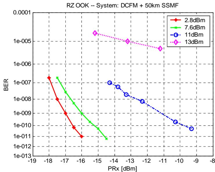
Figure 59 transmission over 50 km SSMF: BER versus Rx sensitivity with total launched power as a parameter. Modulation format: RZ-ASK
