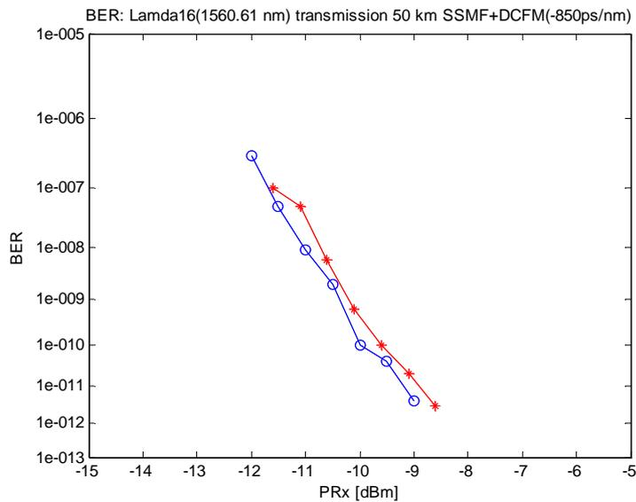
Figure 26 Optical transmission over dispersion managed 50 km of SSMF + DCFM (total dispersion -850 ps/nm); Modulation format = CSRZ –DPSK (red) and RZ-DPSK (blue), Eye diagram captured. Note: full clock recovery used for sampling the EA 44E. Centre wavelength ( $\lambda_{16}$ ) = 1560.61 nm
