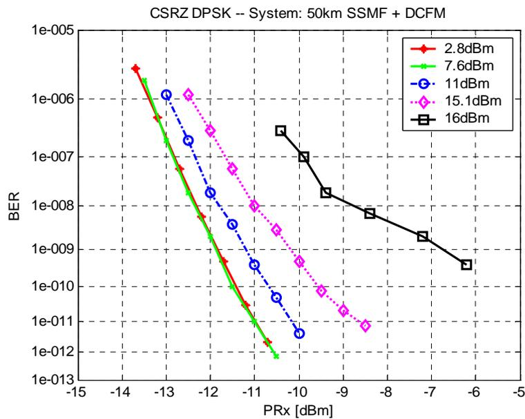
Figure 61 Transmission over 50 km SSMF dispersion management: BER versus Rx sensitivity with total launched power as a parameter. Modulation format: CSRZ-DPSK
