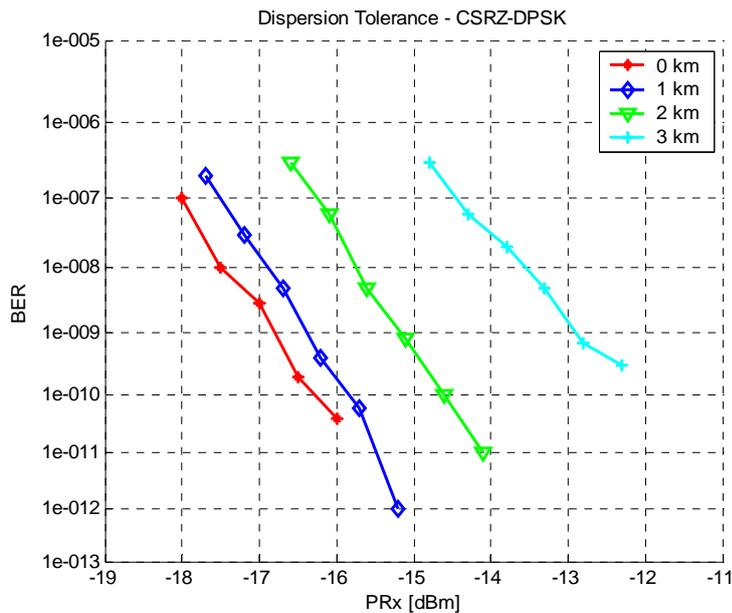
Figure 47 BER as a function of receiver sensitivity with SSMF length as a parameter. Modulation format: carrier-suppressed RZ-DPSK.
