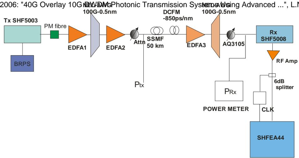
Figure 60 Transmission performance of dispersion managed fibres: 50km SMF + DCF-850
