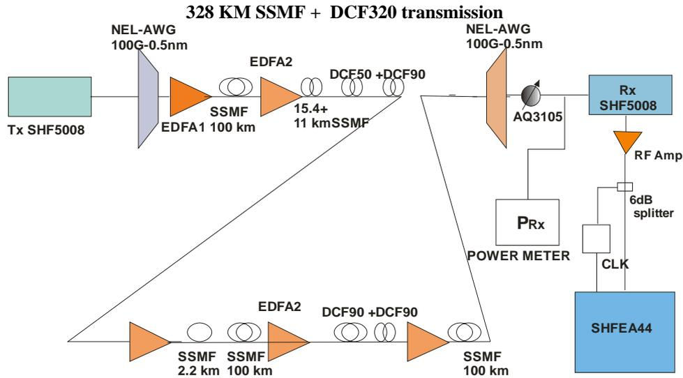
Figure 38 328 KM SSMF + 320 DCF Transmission with CSRZ-DPSK and RZ – DPSK formats Notes: The length of SSMF is selected to be 328 km as it gives the best BER which can be achieved (theoretically, dispersion is nearly completely compensated)
